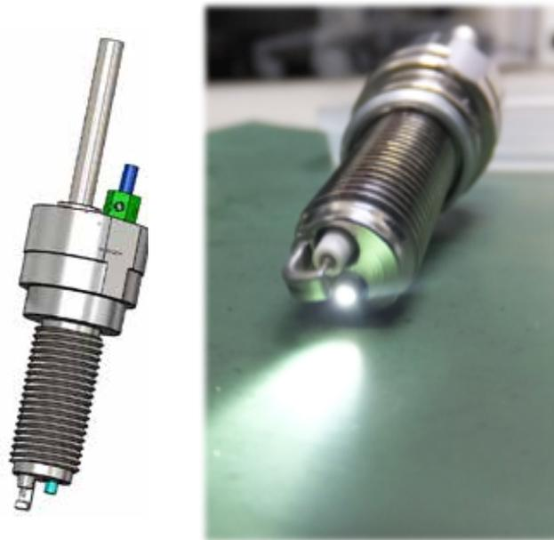
Fig. 2 Spark-plug sensor with optical fiber
