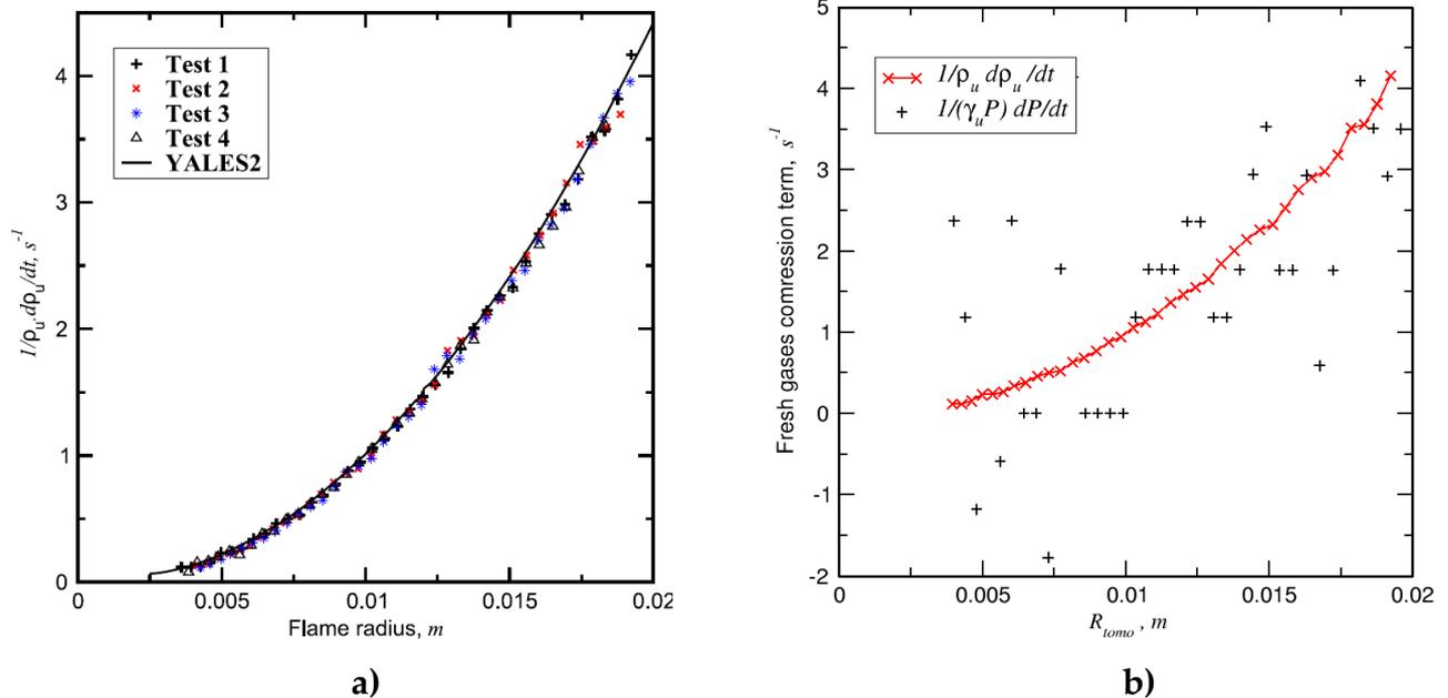
**Fig. 3** Left: Time derivative of the fresh gas density compared to simulation with respect to the experimental flame radius. Right: Comparison between the experimentally determined two terms  $\frac{1}{\rho_u} \frac{d\rho_u}{dt}$  and  $\frac{1}{\gamma_u P} \frac{dP}{dt}$  with respect to the experimental flame radius. Stoichiometric *CH<sub>4</sub>/air* flame at  $T = 300K$  and  $P = 1atm$ .
