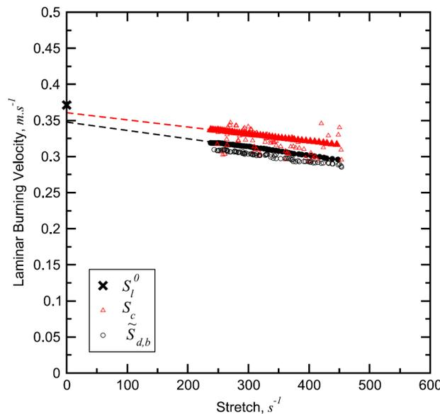
**Fig. 4** Comparison between numerical (filled symbols) and experimental (empty symbols) data of consumptions speed definitions of *CH4=air* flames at atmospheric conditions. The cross at
