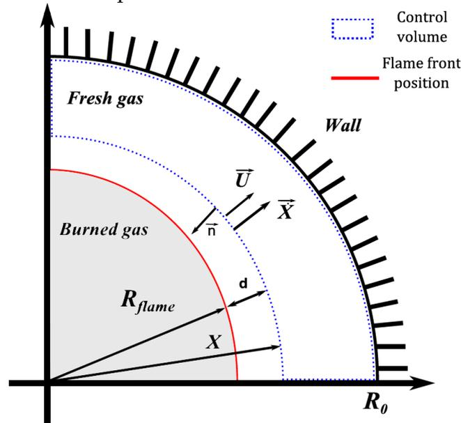
**Fig. 1** Scheme of an infinitely thin flame located at  $R = R_f$  and the temperature and velocity profiles to represent all parameters needed in the present study.
