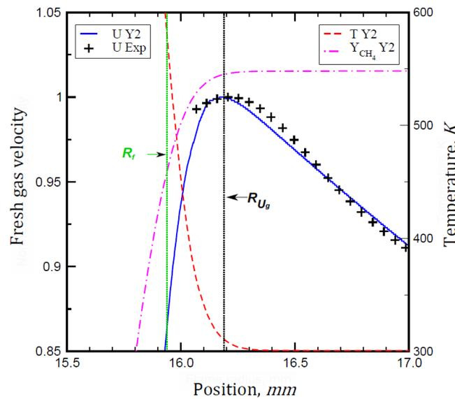
**Fig. 2** Numerical and experimental profiles of normalized fresh gas velocity, temperature and fuel mass fraction of a stoichiometric  $CH_4/air$  flame.  $P = 1atm$ ,  $T = 300K$ . Y2 stands for simulations from YALES2 code.
