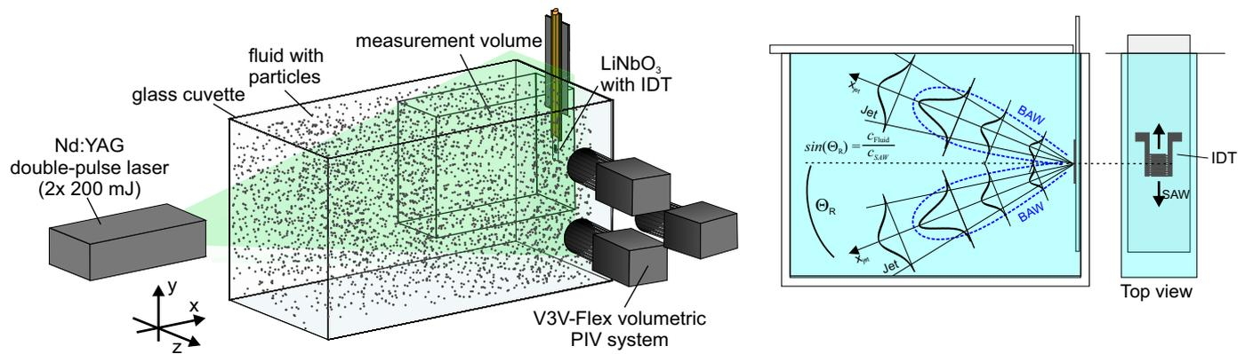
**Fig. 2.** (left) setup used for volumetric particle velocimetry and (right) sketch of the expected BAW and acoustically-induced velocity jets inside the glass cuvette when LiNbO<sub>3</sub> with the IDT is immersed in the fluid
