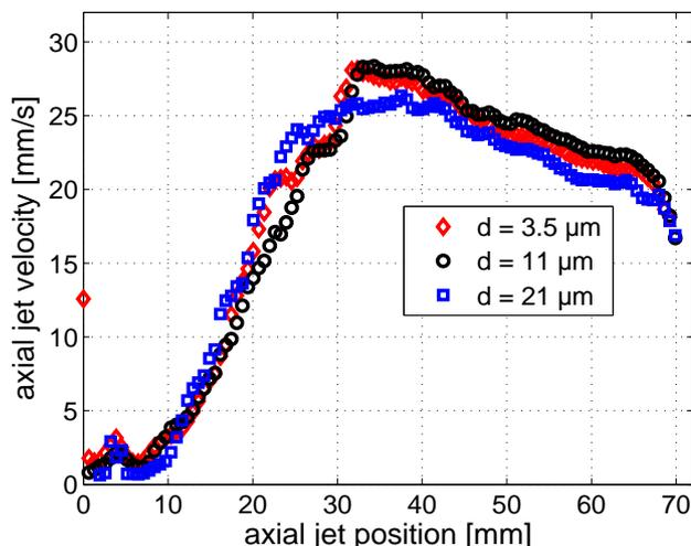
**Fig. 5** Axial jet velocity profile of the lower jet for three different sizes of silver-coated polystyrene particles
