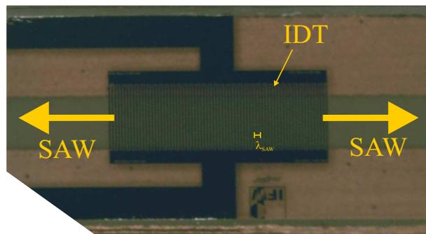
**Fig. 1** Photo of the SAW-device.
