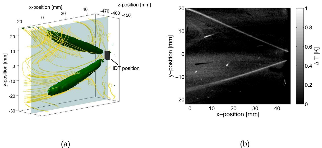
Fig. 4 (a) measured volumetric velocity field and (b) temperature field at the center z position induced by a SAW when an electrical power level of about 7 mW is applied.;  $\Delta T = T_{OFF} - T_{ON}$
