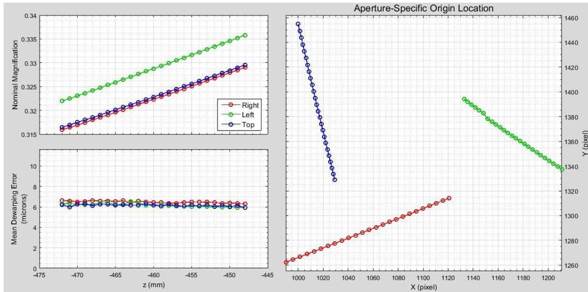
**Fig. 3:** Calibration result of the V3V-Flex system with 3 cameras.
