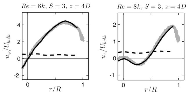
**Fig. 2** Comparison between LDA and PC-MRI for a selected configuration. The gray lines represent the circumferentially averaged velocity profiles from PC-MRI. The solid black lines denote the LDA data and the dashed lines represent the corresponding RMS values from the LDA measurements.
