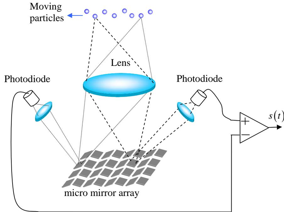
Figure 3.6: Principle of micro mirror array for spatial filtering velocimetry (shown: differential grating)
