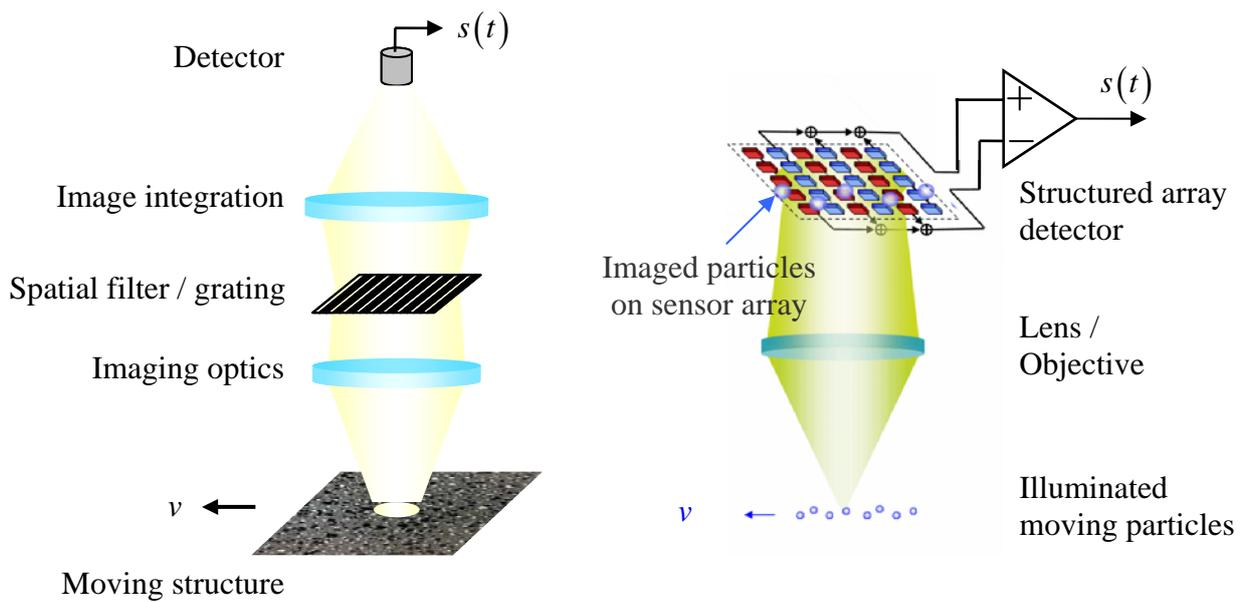
Figure 2.1: a) left: Spatial filtering system with hardware grating, b) right: implementation of a differential grating using structured array detectors.
