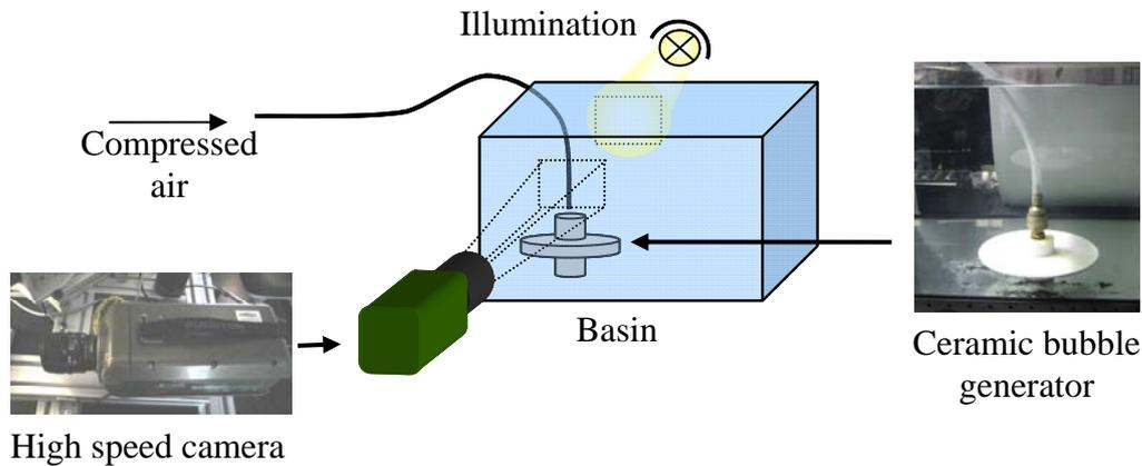
Figure 3.1: Measurement setup for observing bubbles in a water basin
