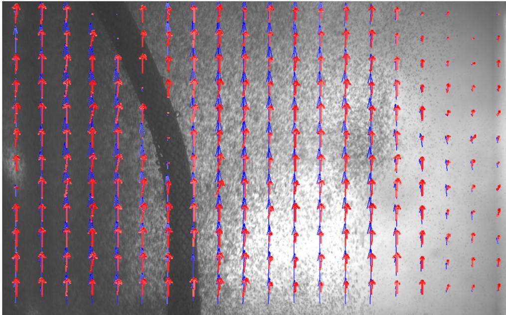
Figure 3.2: Observed bubbles in the water basin (blue arrows: mean of 1024 cross-correlation results, red arrows: results of same sequence using the PSD peak of spatial filtering signals)
