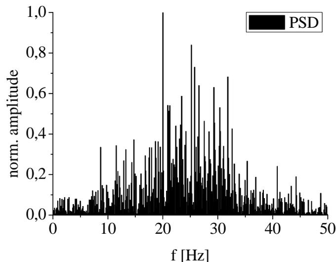
Figure 3.3: PSD of spatial filtering signal in vertical direction
