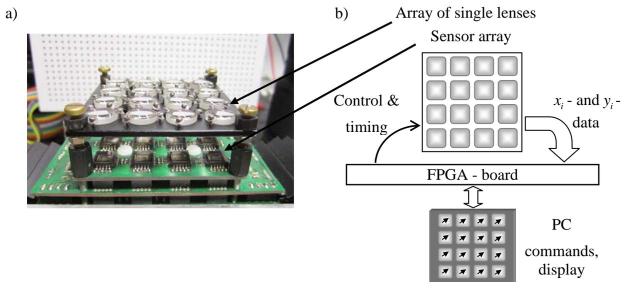
Figure 3.4: Sensor array of smart pixel sensors (a: picture of the sensor array, b: schematic configuration of array sensor)
