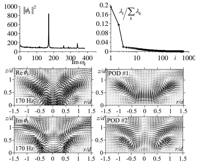
**Fig. 2** Spectra and spatial distributions of the most powerful modes for (left) DMD and (right) POD in a forced at 170 Hz propane-air lifted flame.
