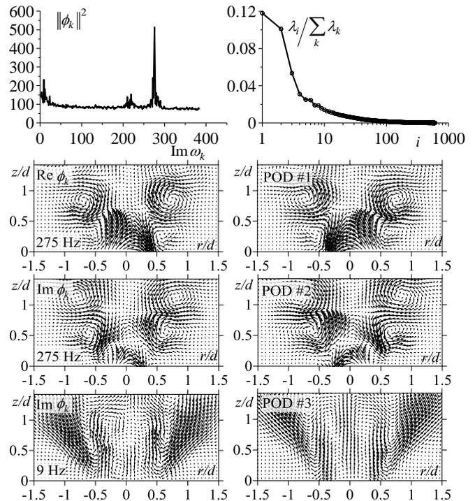
**Fig. 1** Normalized spectra and spatial distributions of the most powerful modes for (left) DMD and (right) POD in an unforced propane-air lifted flame.
