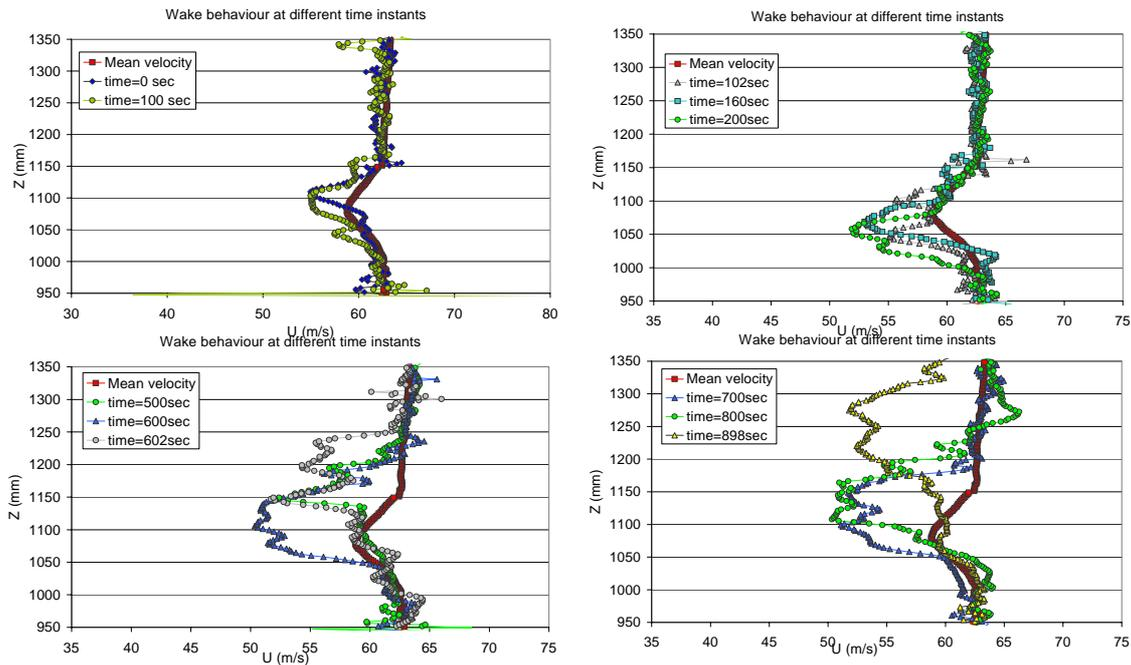
**Figure 20: Wake behavior at different time instant during ice accretion**
