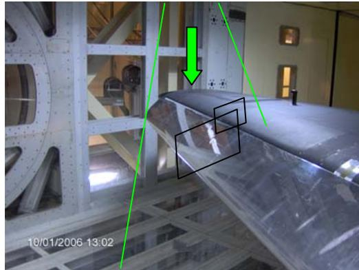
**Figure 9: PIV recording set up on the LE**
