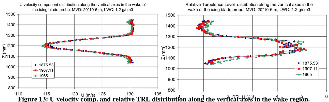
**Figure 13: U velocity comp. and relative TRL distribution along the vertical axes in the wake region.**
