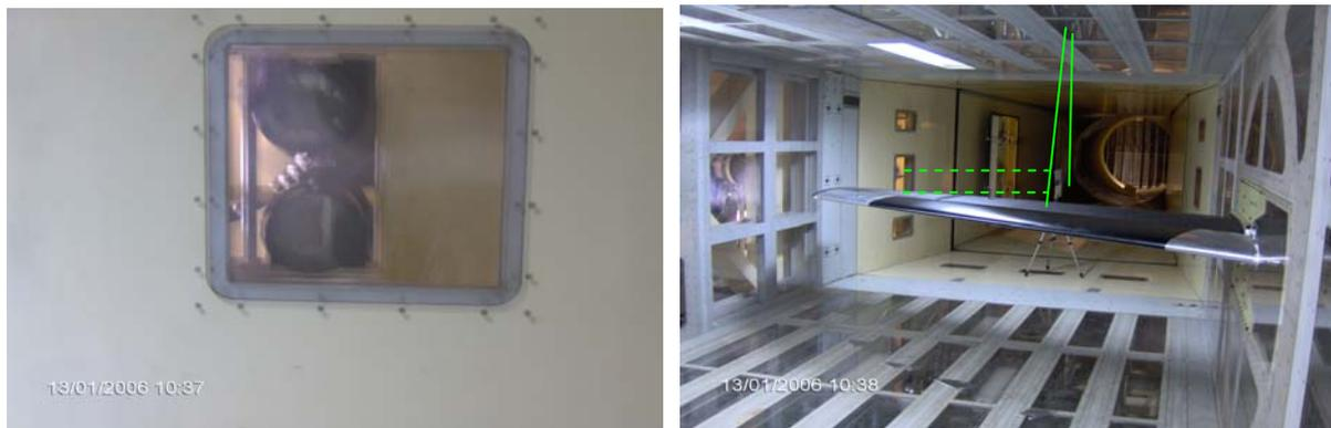
**Figure 10: Recording camera and experimental set up in the wake region**
