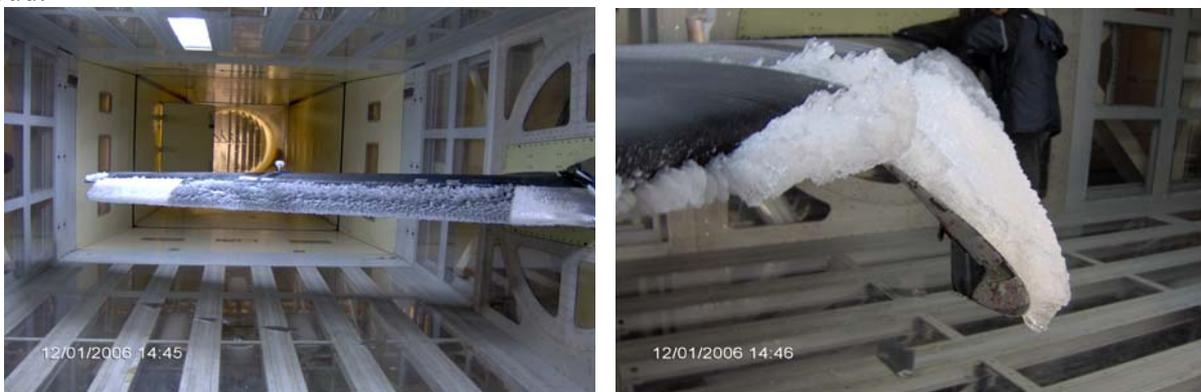
Figure 18: Front and side view of the wing after the accretion of the ice
