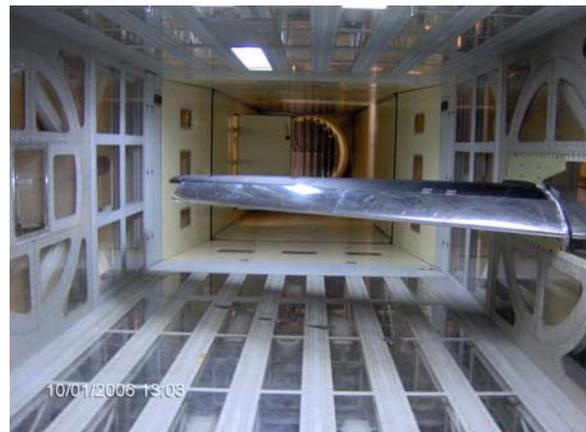
Figure 3: Swept wing mounted in the additional TS
