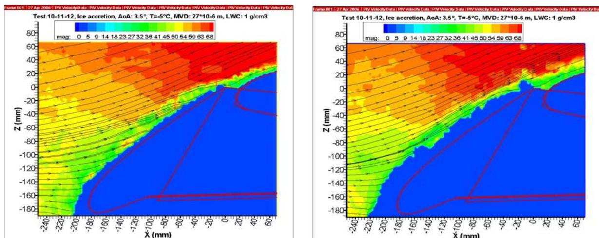
Figure 19: PIV results obtained respectively after 5 and 15 minutes from the start of the ice accretion.
