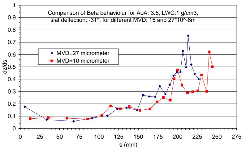
Figure 16: Collection efficiency versus surface coordinate.
