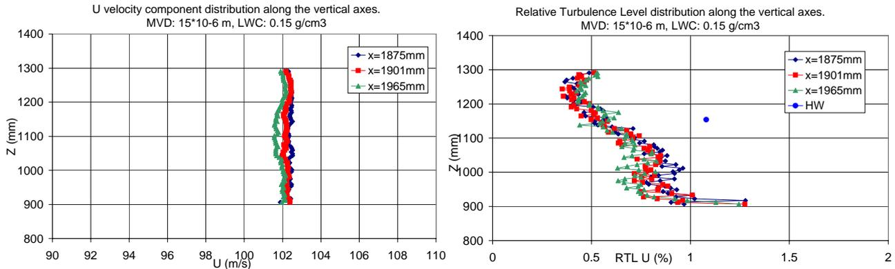
**Figure 11: U velocity comp. and RTL distribution along the vertical axes in free stream condition.**
