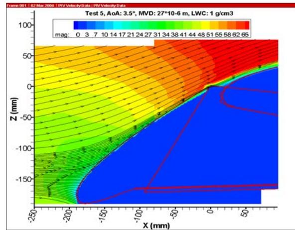
Figure 15: Droplet trajectories and velocity field colour map
