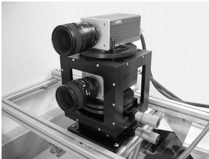
Fig. 4. Two synchronized two-component PIV cameras arrangement.
