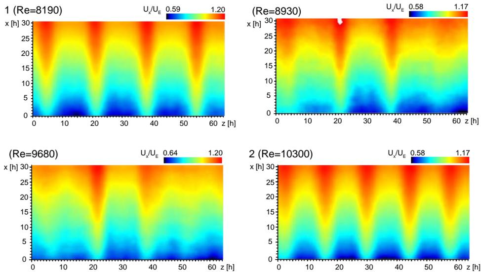
Fig. 8. Selected mean-velocity fields showing the effect of Reynolds number.
