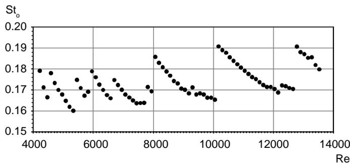
Fig. 7. Non-dimensional vibration frequency ( $St_0$ ) as a function of the Reynolds number.
