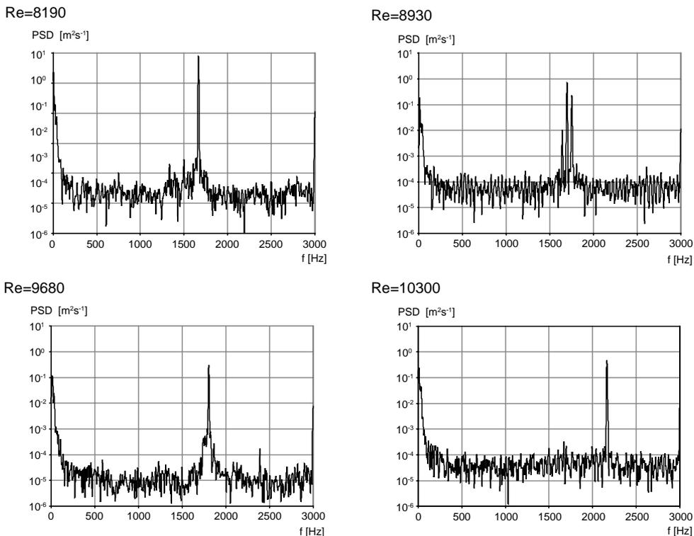
Fig. 9. Tip vibration spectra measured with HSDI corresponding to Reynolds numbers in Fig. 8.
