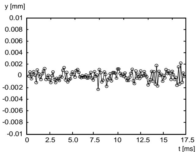
Fig. 4. An example of the time-trace of low amplitude vibration with stainless steel plate.
