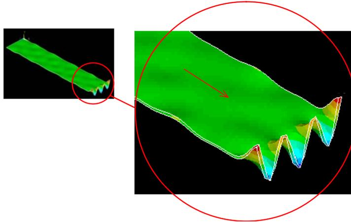
Fig. 5. A snapshot from computational modal analysis showing a standing vibration mode.
