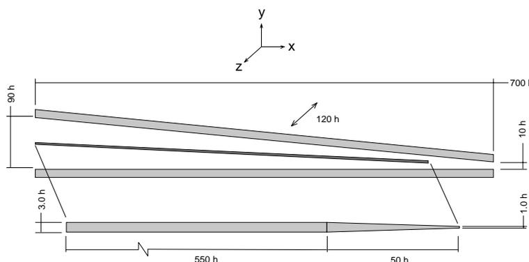
Fig. 1. Dimensions of the flow channel and the splitter plate.
