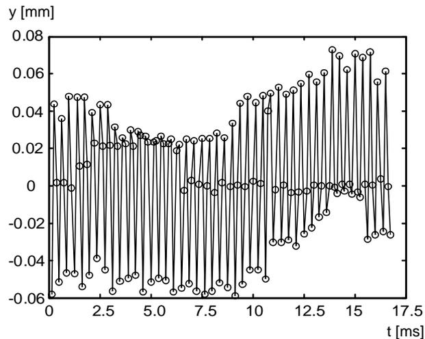
Fig. 3. An example of the time-trace of the tip  $y$ -position detected by HSDI.
