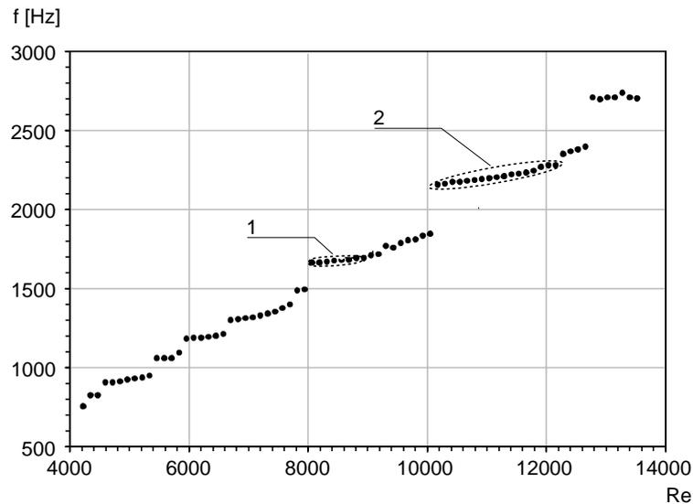
Fig. 6. Vibration frequency of the plate tip as a function of Reynolds number.
