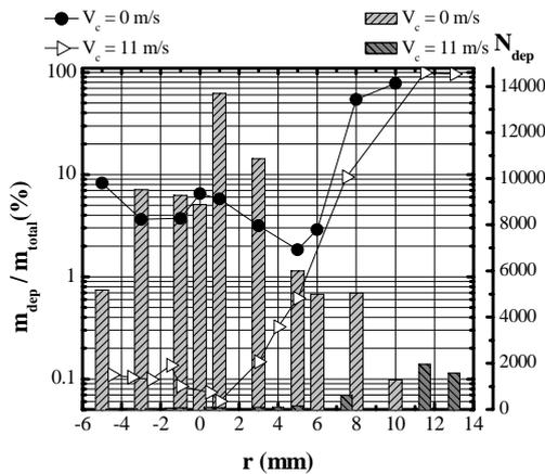
**Fig. 9** Fraction from the mass of all droplets that crossed the PDA measurement volume expected to deposit on the wall.
