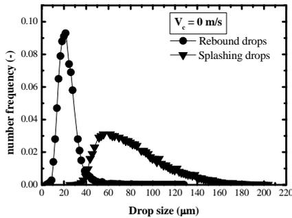
**Fig. 10** Size distributions of impinging drops predicted to contribute for secondary atomization ( $-5 \leq r \leq 10$  mm).
