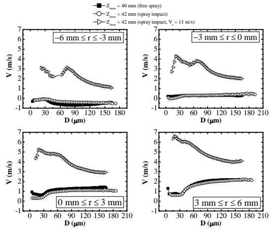
Fig. 8 Drop size-radial velocity correlation at four regions of the spray.
