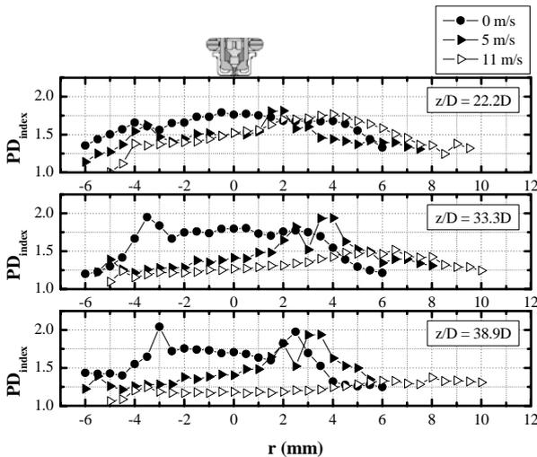
**Fig. 5** Polydispersion degree index ( $PD_{index} = SMD/AMD$ ) below the injector nozzle at 7 ms ASOI, with and without cross-flow for 22.2D, 33.3D and 38.9D, with  $D = 0.9$  mm.
