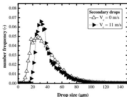
**Fig. 13** Size distributions of droplets produced by secondary atomization under quiescent surroundings ( $-5 \leq r \leq 10$  mm) and in the presence of an 11 m/s cross-flow ( $-5 \leq r \leq 14$  mm).
