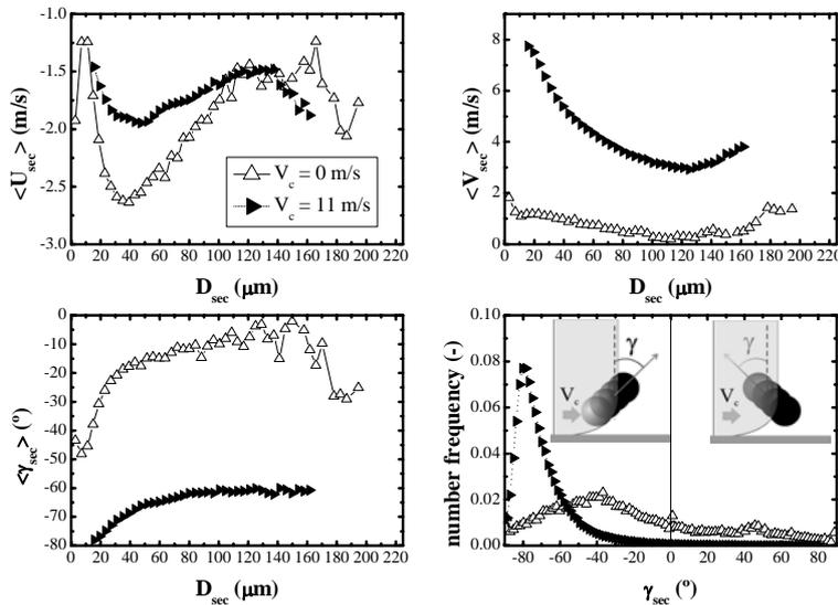
**Fig. 15** ‘Ensemble-average’ axial velocity ( $\langle U_{sec} \rangle$ ), radial velocity ( $\langle V_{sec} \rangle$ ), direction ( $\langle \gamma_{sec} \rangle$ ) – drop size correlations, and discrete direction distributions, for secondary droplets under quiescent surroundings ( $-5 \leq r \leq 10$  mm) and in the presence of an 11 m/s cross-flow ( $-5 \leq r \leq 14$  mm).
