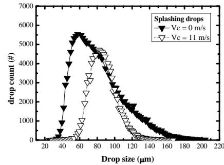
**Fig. 11** Size distributions of impinging drops predicted to splash under quiescent surroundings ( $-5 \leq r \leq 10$  mm) and in the presence of an 11 m/s cross-flow ( $-5 \leq r \leq 14$  mm).
