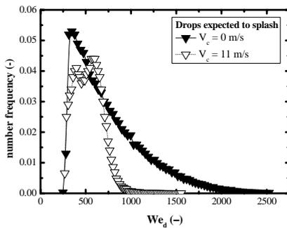
**Fig. 12** Discrete probability distributions of the Weber number of drops predicted to splash under quiescent surroundings ( $-5 \leq r \leq 10$  mm) and in the presence of an 11 m/s cross-flow ( $-5 \leq r \leq 14$  mm).
