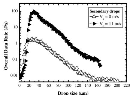
**Fig. 14** Overall data rate as a function of drop size of secondary droplets under quiescent surroundings ( $-5 \leq r \leq 10$  mm) and in the presence of an 11 m/s cross-flow ( $-5 \leq r \leq 14$  mm).
