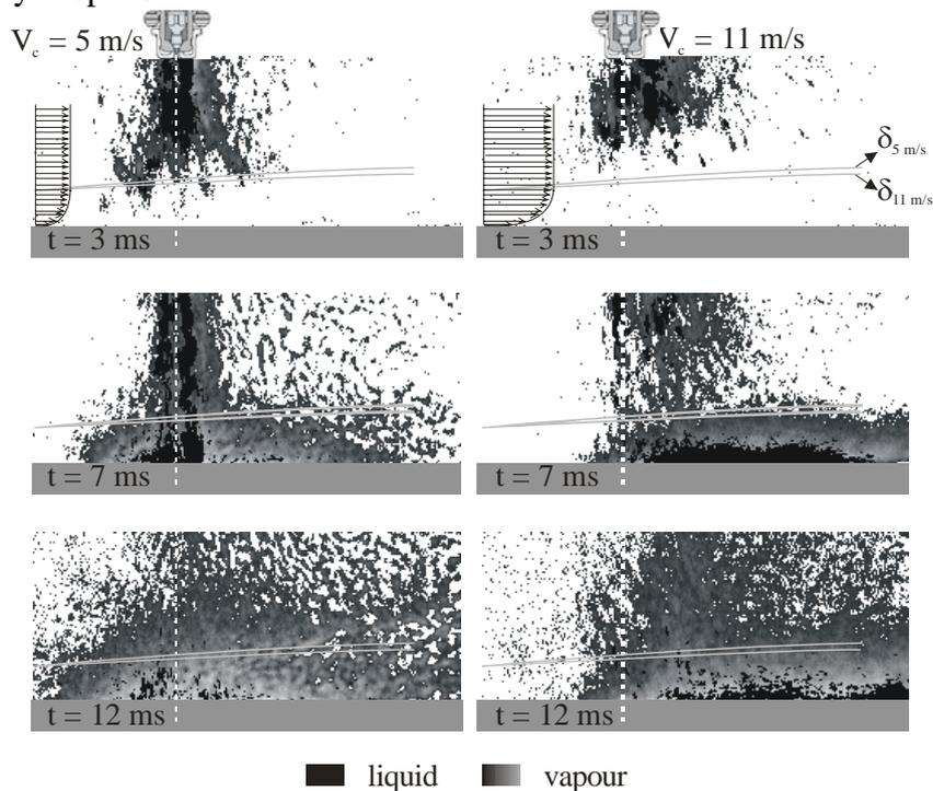
**Fig. 3** Combined Mie scattering and shadowgraph images of spray impact for two different cross-flow velocities.
