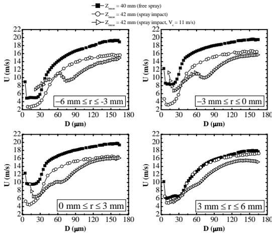
Fig. 7 Drop size-Axial velocity correlation at four regions of the spray.
