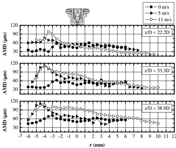
**Fig. 4** Arithmetic mean diameter below the injector nozzle at 7 ms ASOI with and without cross-flow at 22.2D, 33.3D and 38.9D, with  $D = 0.9$  mm.
