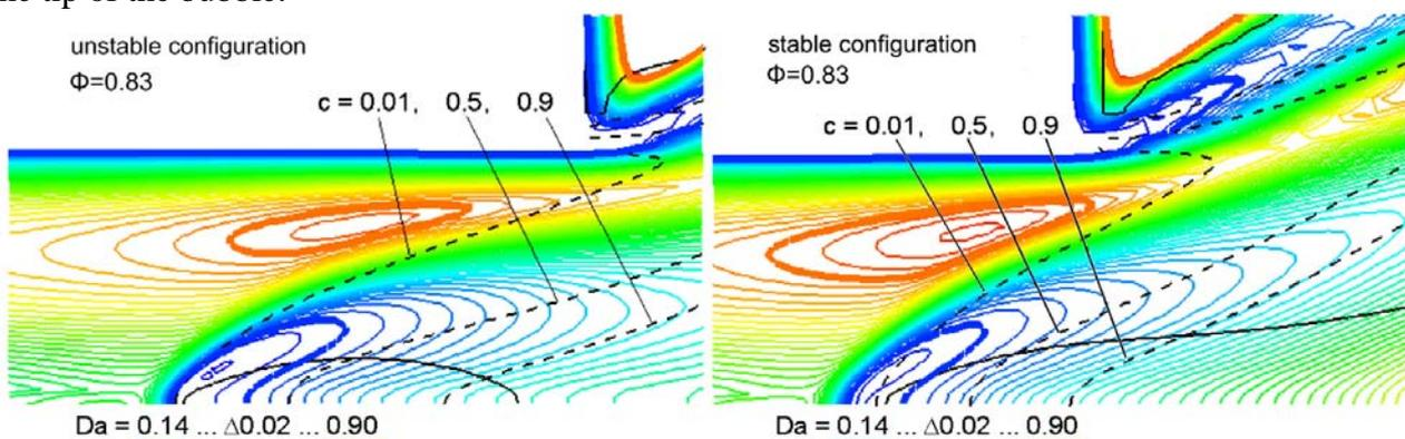
**Fig. 2** Numerical comparison of the Da distribution for a safe as well as a CIVB prone configuration (Kiesewetter 2005).
