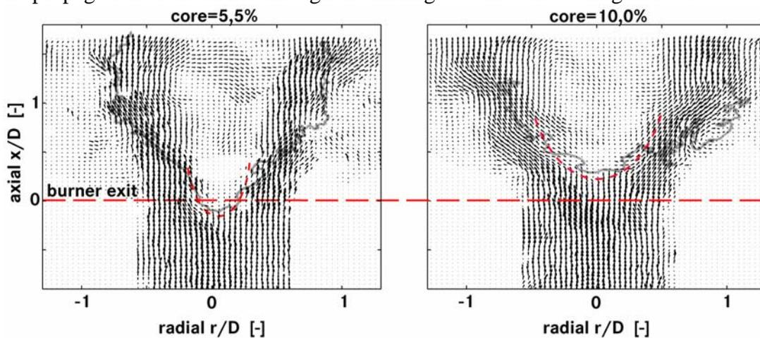
**Fig. 10** Influence of the core flow on the bubble position
