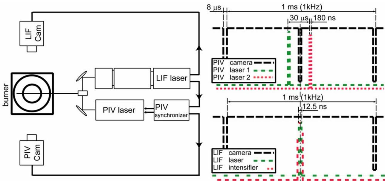
Fig. 7 Sketch of the setup and the triggering scheme
