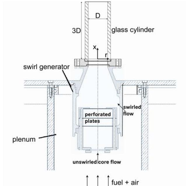
Fig. 5 Sketch of the investigated burner system
