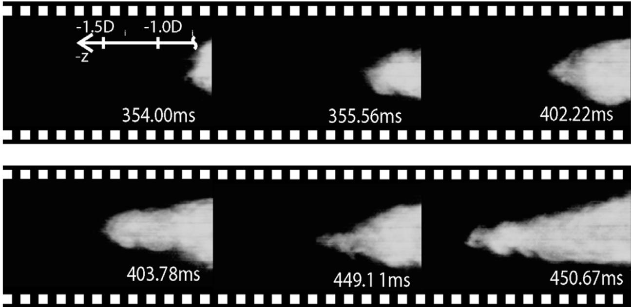
**Fig. 1** Flame propagation during a CIVB driven flashback (Fritz et al. 2004).
