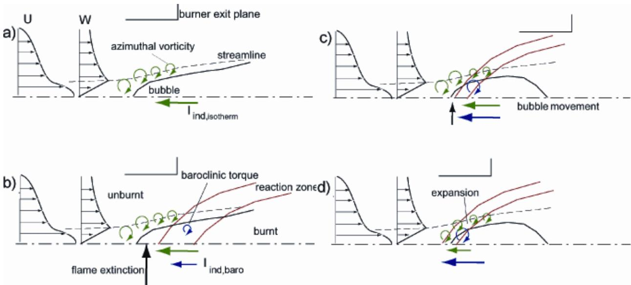
**Fig. 4** The principle of the new understanding of CIVB driven flashbacks.
