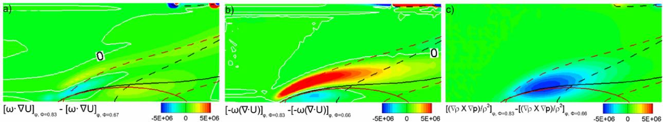
**Fig. 3** Numerical calculation of the influence of the equivalence ratio on the source terms of the vorticity transport equation (stretching/tilting (a), volumetric expansion (b) and baroclinic torque (c)) (Kiesewetter 2005).
