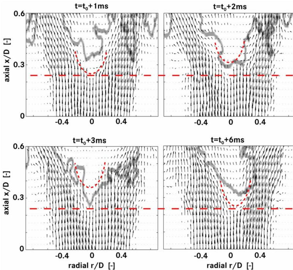
**Fig. 9** Behavior of the bubble during flame propagation
