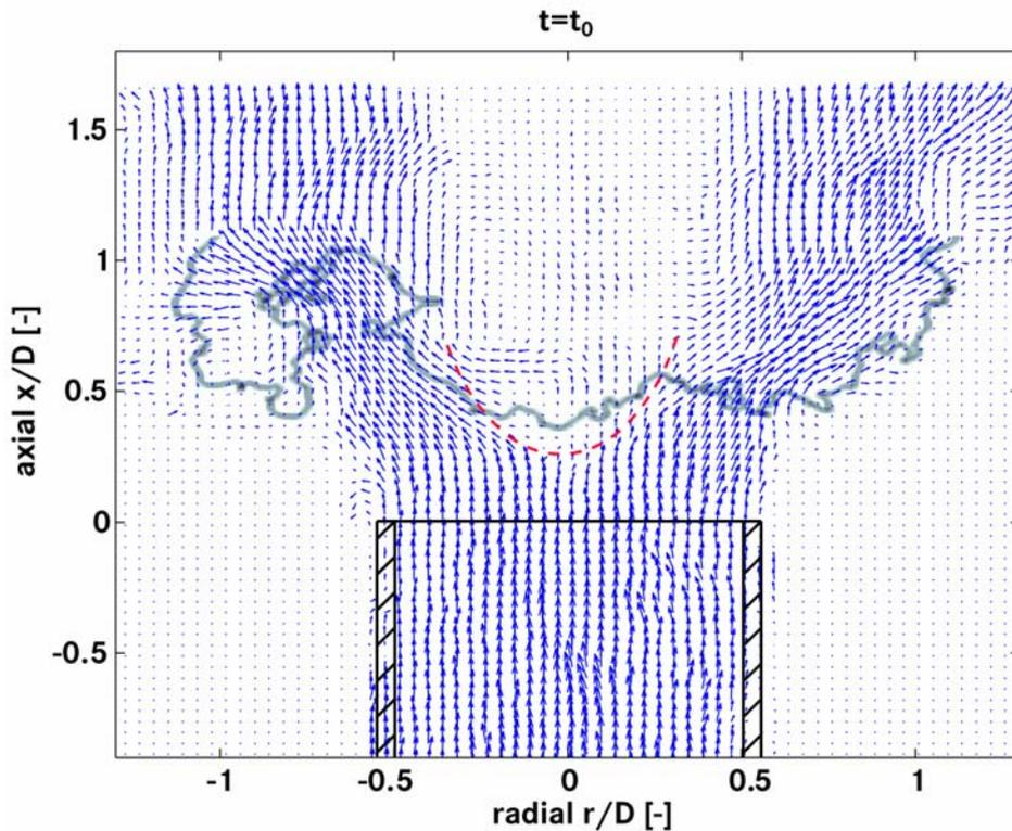
**Fig. 8** Flame front (gray line) and velocity field (vectors); the bubble envelope is shown with a dotted curve
