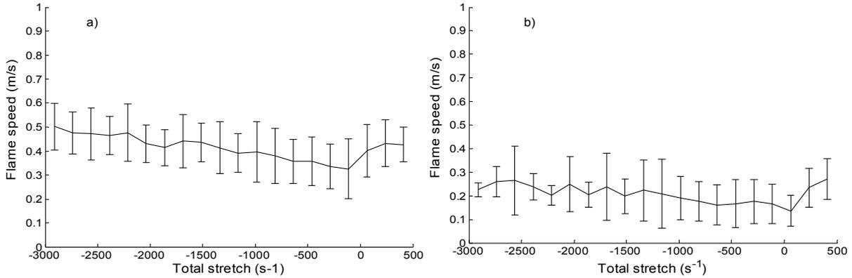
Fig. 5. Flame speed variation variation relative to total flame stretch. Premixed propane/Air with equivalence ration a)  $\Phi=0,86$  and b)  $\Phi=1,52$
