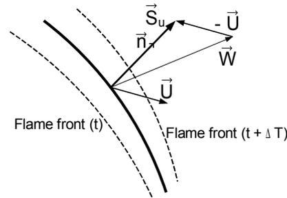
Fig. 1. Velocity triangle in the flame front
