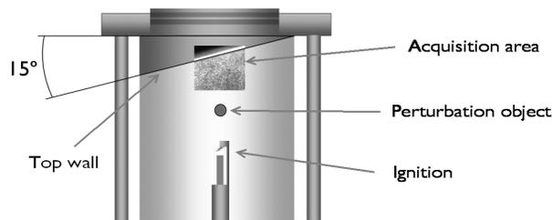
Fig. 3. Combustion chamber detail of flame wall interaction region
