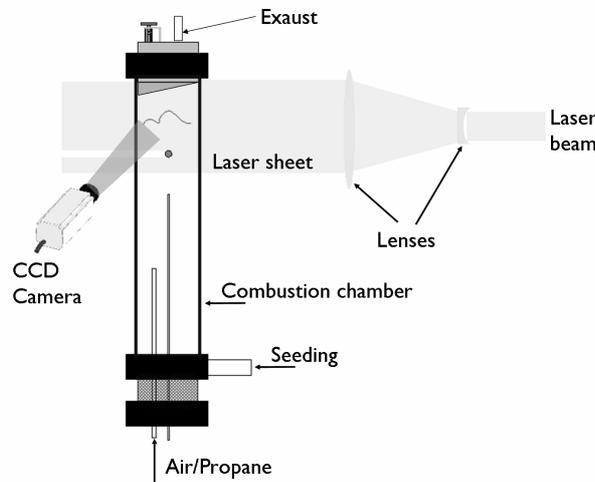
Fig. 2. Installation setup for image acquisition
