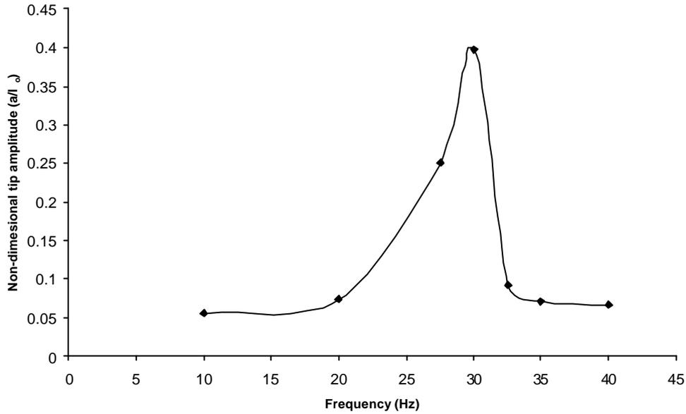
**Figure 3.** Tip amplitude deviation with varying frequency at largest applied voltage (150V)
