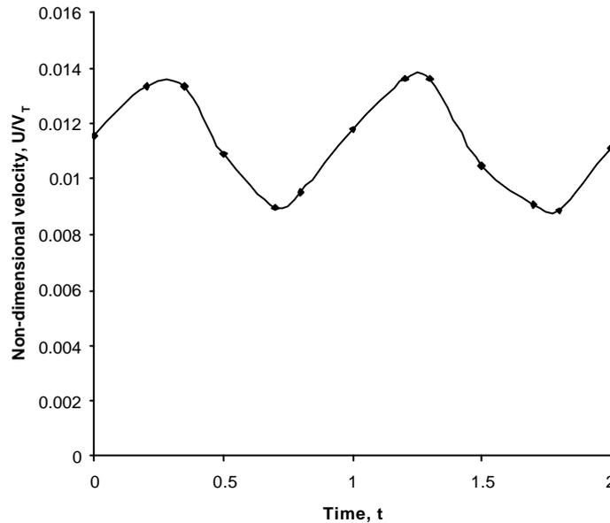
**Figure 11.** Velocity variation for a given point throughout the oscillation
