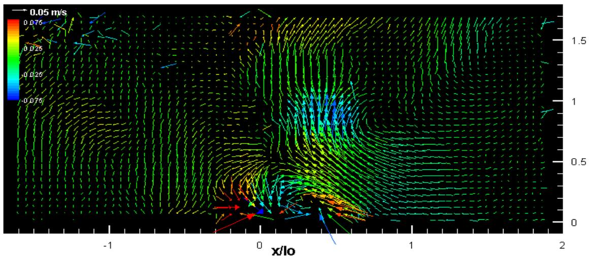
Figure 10b Instantaneous vector plot for  $a/l_0 = 0.397$  ( $Re_a = 0.1777$ )
