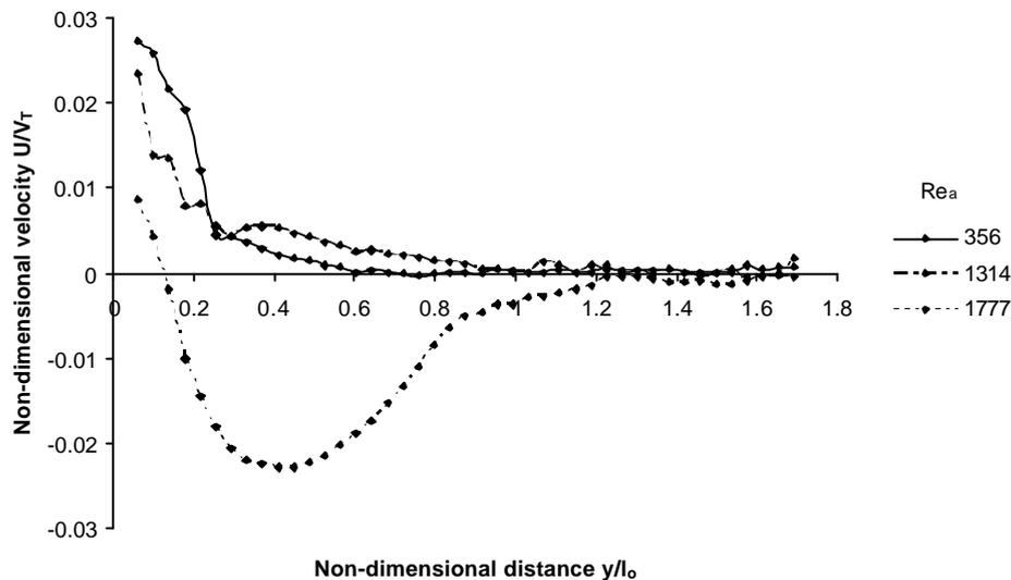
**Figure 9.** Centreline velocity distribution for the three amplitudes
