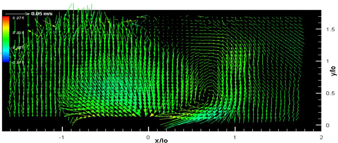
Figure 6. Time averaged vector plot for  $a/l_0 = 0.340$ ,  $Re_a = 1314$
