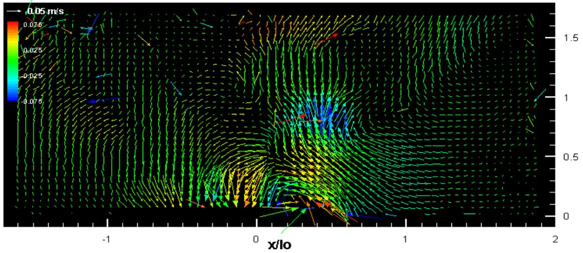
Figure 10a. Instantaneous vector plot for  $a/l_0 = 0.397$  ( $Re_a = 0.1777$ )
