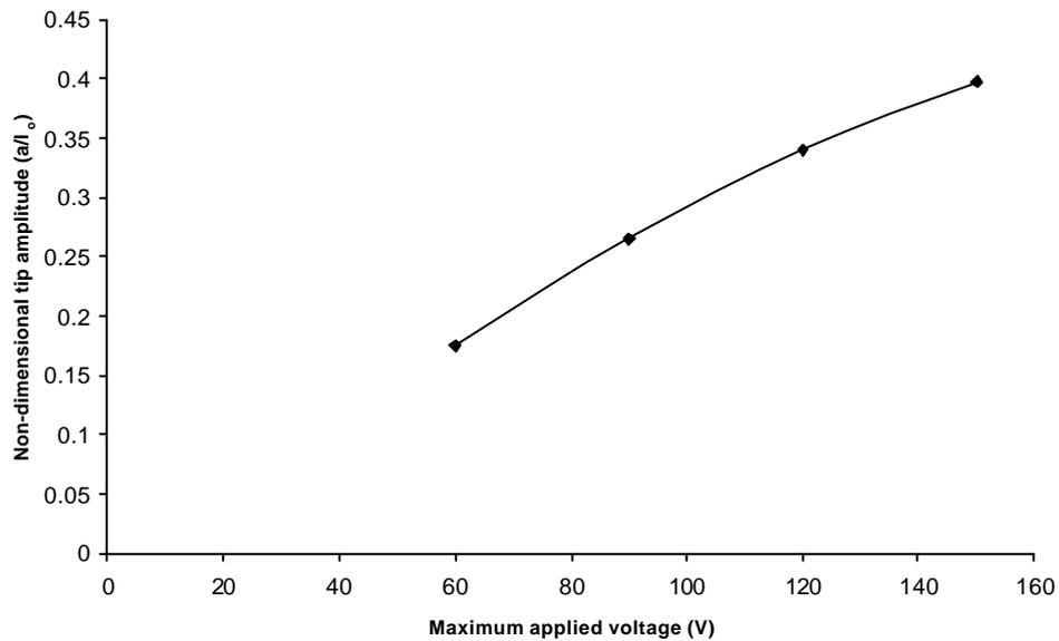
**Figure 4.** Variation of tip amplitude with applied voltage at resonant frequency (30Hz)
