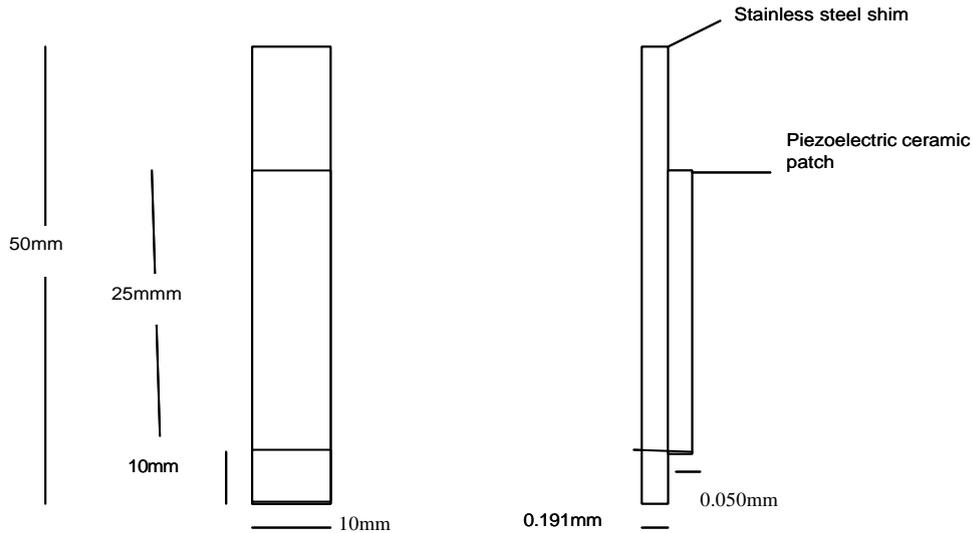
**Figure 1.** Details of the pie zoelectric unimorph
