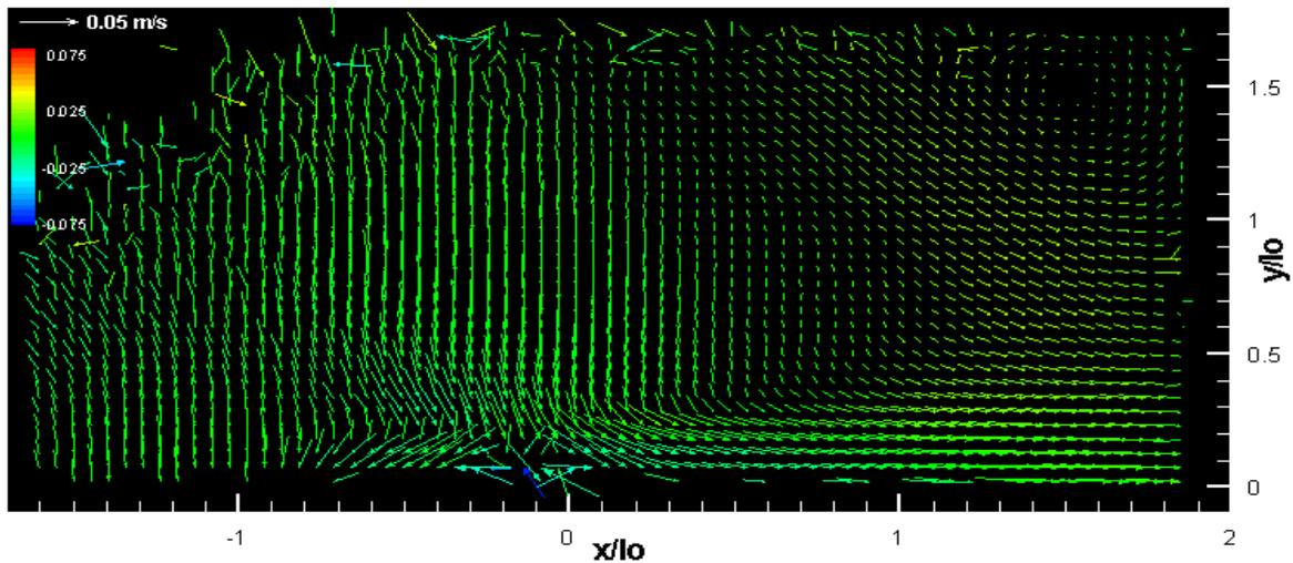
Figure 5. Time averaged vector plot for  $a/l_0 = 0.176$ ,  $Re_a = 356$
