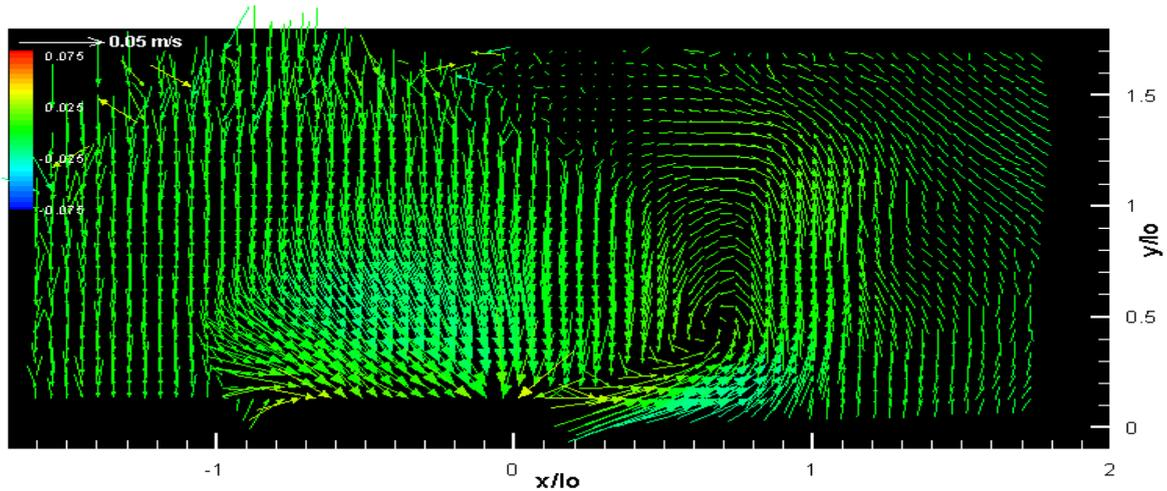
**Figure 7.** Time averaged vector plot for  $a/l_0 = 0.396$ ,  $Re_a = 1777$
