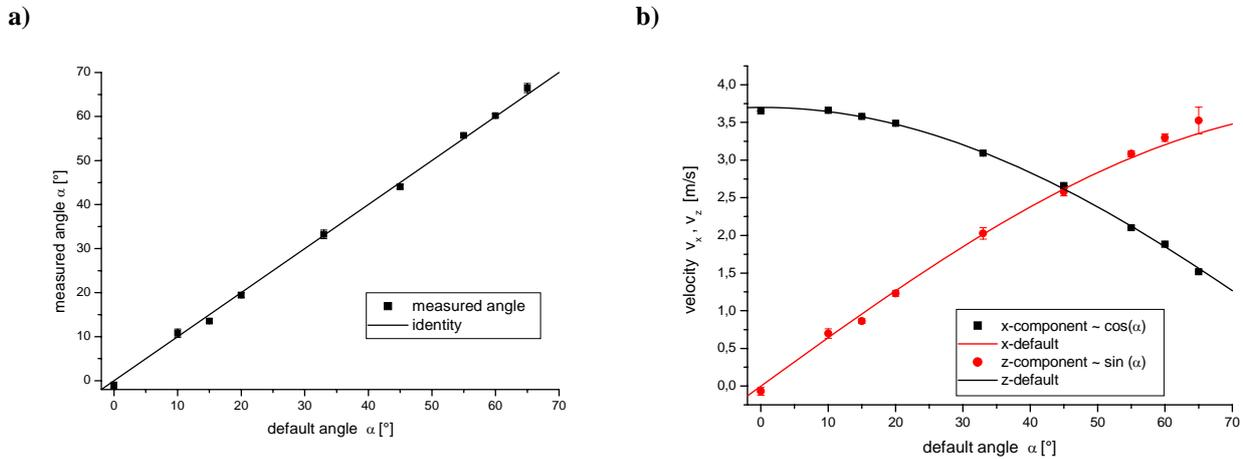
**Fig. (8): Test of a) the angle and b) the velocity component measurement for different inclination angles of a calibration object. An excellent agreement between the default and the measured values occurs.**
