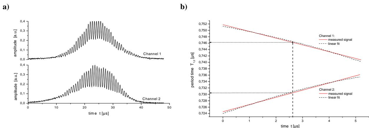
**Fig. (7):** a) Chirped burst signal pair from a particle passing with  $\alpha=30^\circ$  to the optical axis. b) Period time – time functions for both channels, obtained from the short-time FFT. The momentary values at the marked point of time are used to calculate the offset position  $z_0$  and the lateral velocity component  $v_x$ , whereas the slope of the functions yields the axial  $v_z$ -component.
