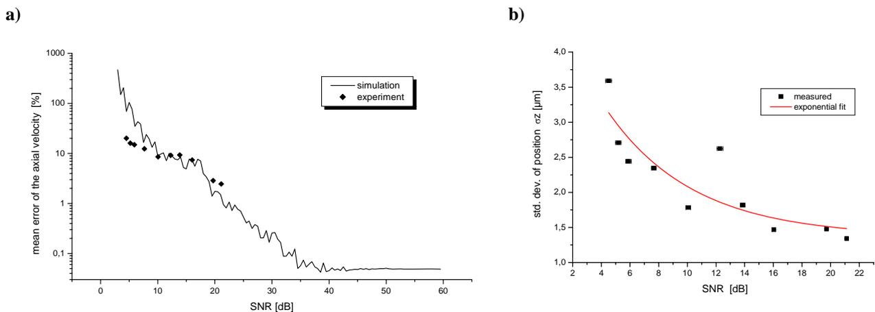
**Fig. (9): Uncertainty estimation of a) the axial velocity component  $v_x$  (solid: simulation, dotted: experiment) and b) of the offset position  $z_0$  (dotted: measurement, solid: exponential fit) in dependence from the SNR.**
