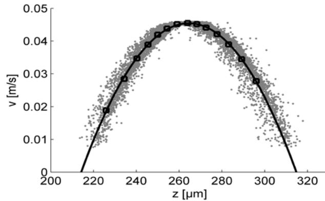
**Fig. (5): Measured velocity profile inside a micro-channel of 100 μm width (solid line: fitted parabolic curve).**
