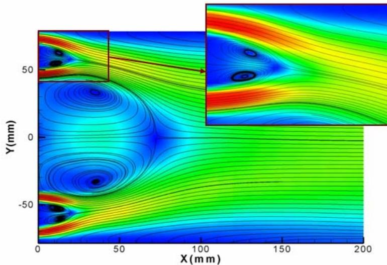
Figure 5 Averaged Velocity Magnitude (Colour Contours) and streamlines
