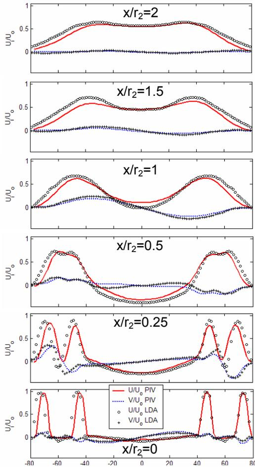
Figure 12 Comparison of PIV and LDA:
