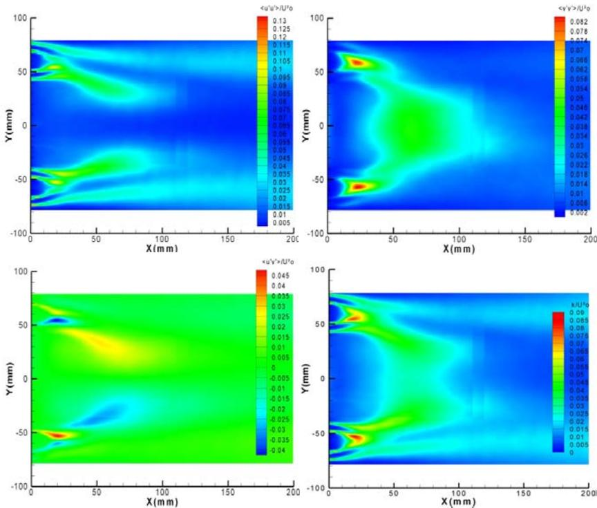
Figure 7 Reynolds stress components and turbulent kinetic energy
