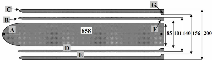
Figure 1 Double annular burner geometry with major dimensions in mm
