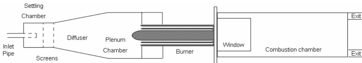
**Figure 3 Complete experimental configuration**
