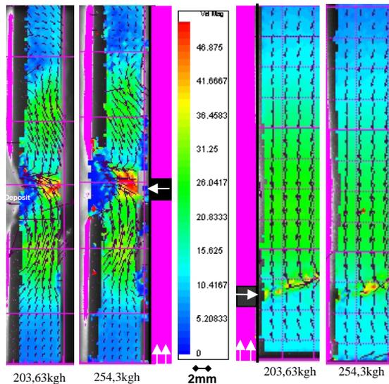
Fig. 12. Mean velocity field near the breach for the jet in tube bundle and for free jet
