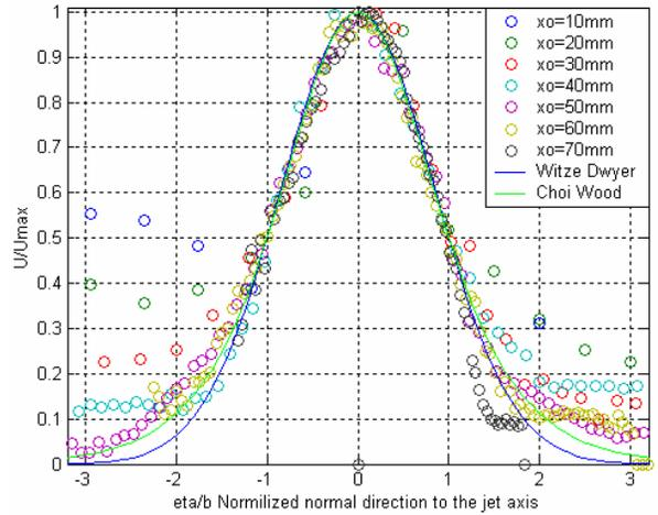
Fig. 9. Velocity profiles measured along the jet center line for different radial distances to the breach. 107 kg/h case
