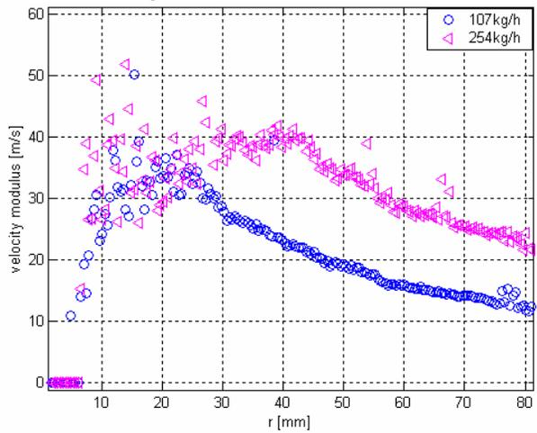
Fig. 11. Maximum jet velocity evolution with the radial distance to the breach
