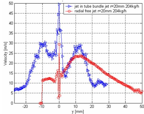
Fig. 13. Vertical profiles for the velocity modulus near the breach for the jet in tube bundle and for free jet
