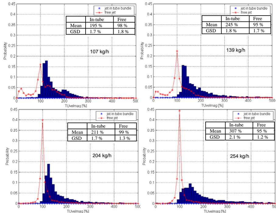
Fig. 14. Tu PDFs comparison for different mass flow rates for jet in tube bundle and free jet
