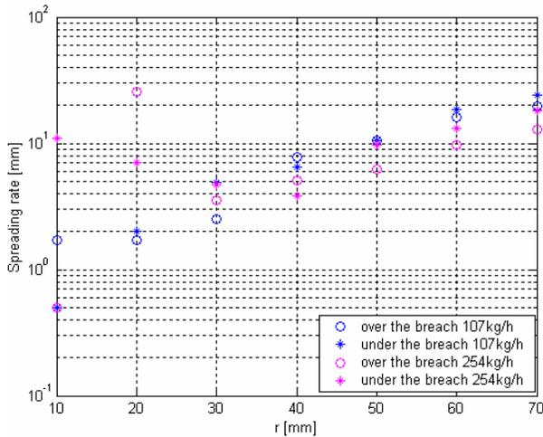
Fig. 10. Spreading rate evolution with the radial distance to the breach
