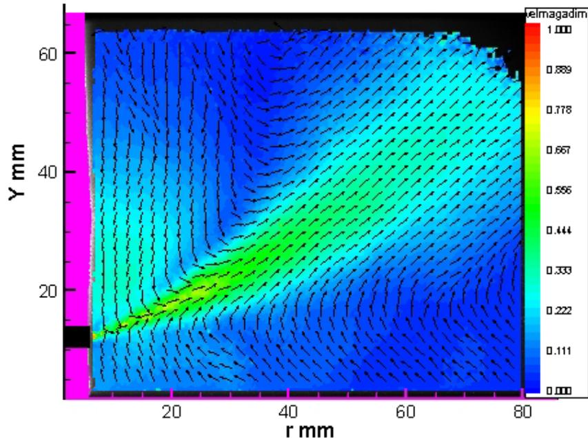
Fig. 7. Normalized mean velocity field for 107 kg/h free radial jet
