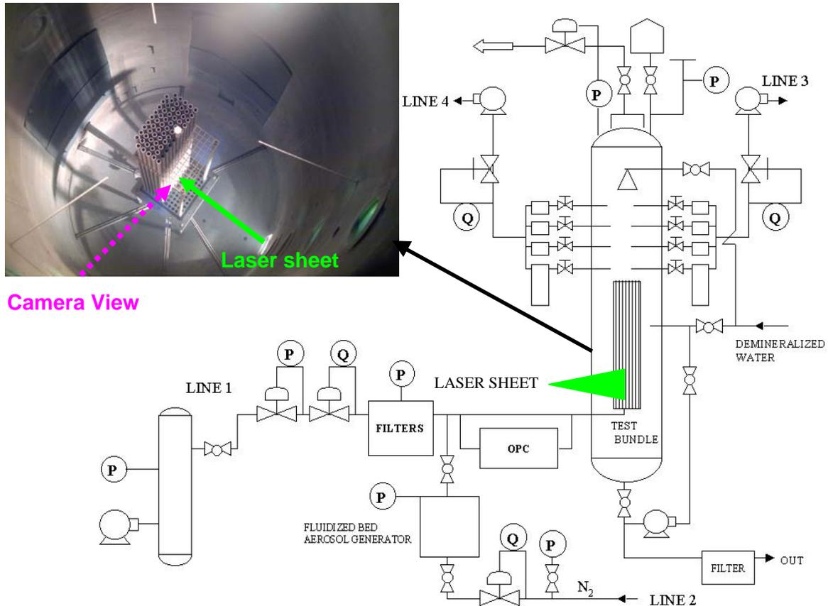
Fig. 1. Scheme of the PECA facility and bundle configuration in the vessel
