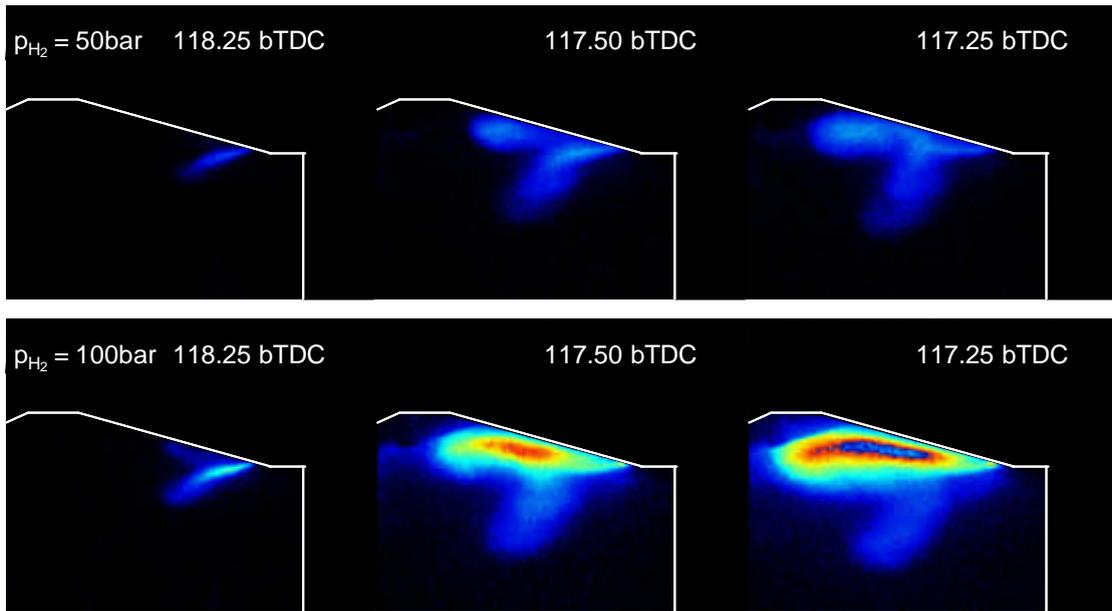
Figure 6: Application of non-quantified LIF-measurements: Comparison of jet patterns for variations of fuel pressure
