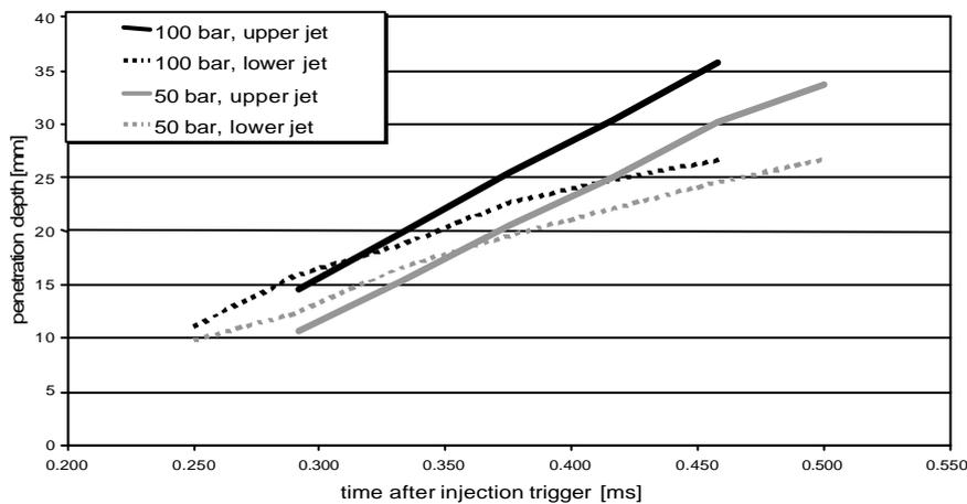
Figure 7: Measurement of intrusion depths
