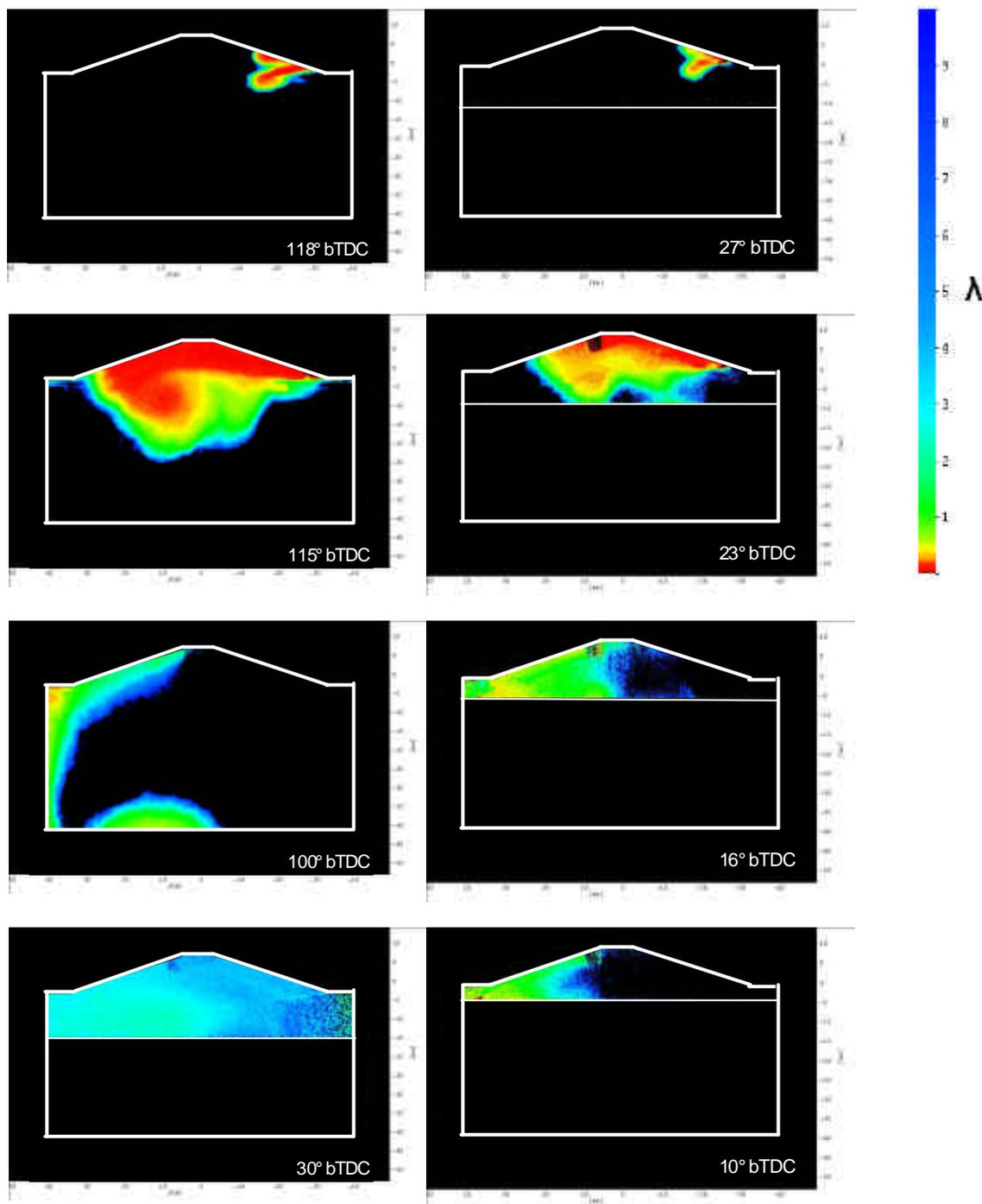
Figure 8: Typical application of quantified LIF-measurements: Comparison of early (left) and late (right) injection
