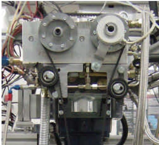
Figure 3: Single-cylinder research engine with optical access into the combustion chamber
