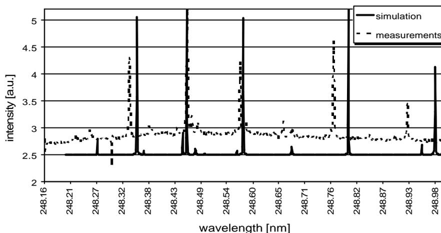
Figure 2: Simulated (LIFBase) and measured LIF-excitation spectrum of the OH-radical
