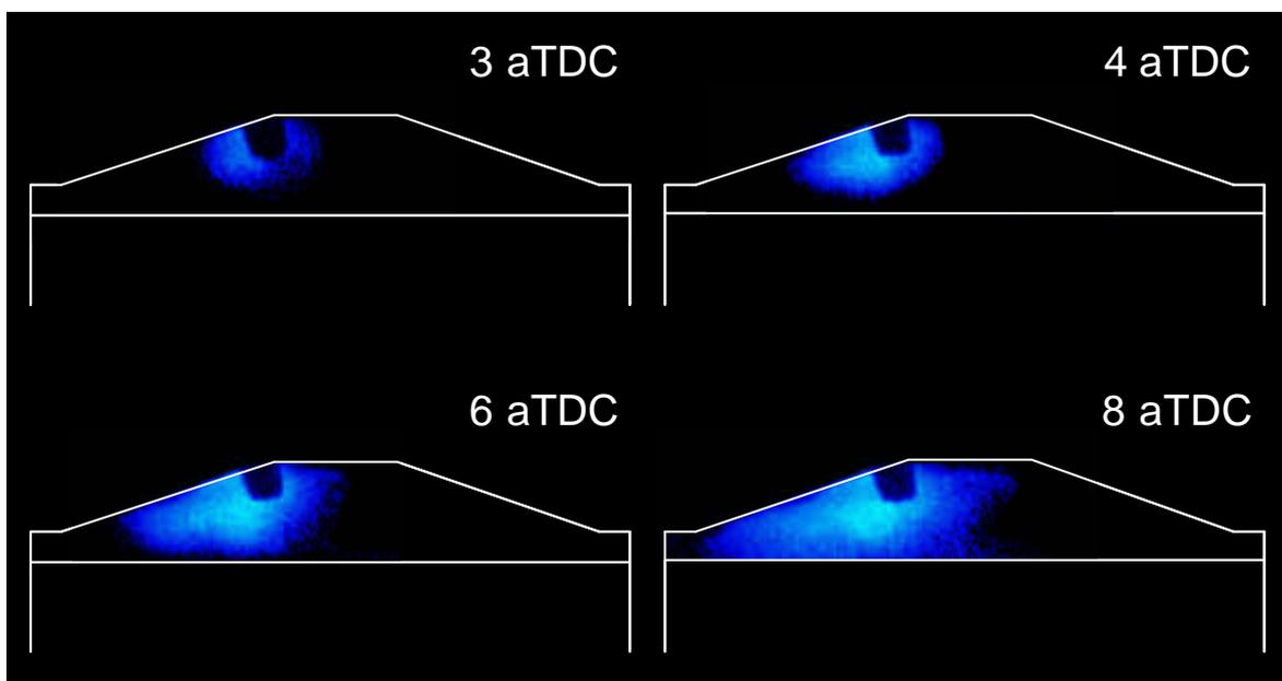
Figure 9: Application of combustion analysis: Visualization of flame propagation for non-homogeneous charges
