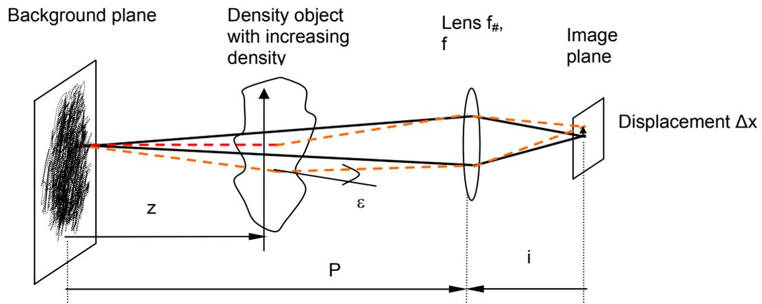
**Figure 1: BOS set up:** z: Distance between the background plane and density object;
