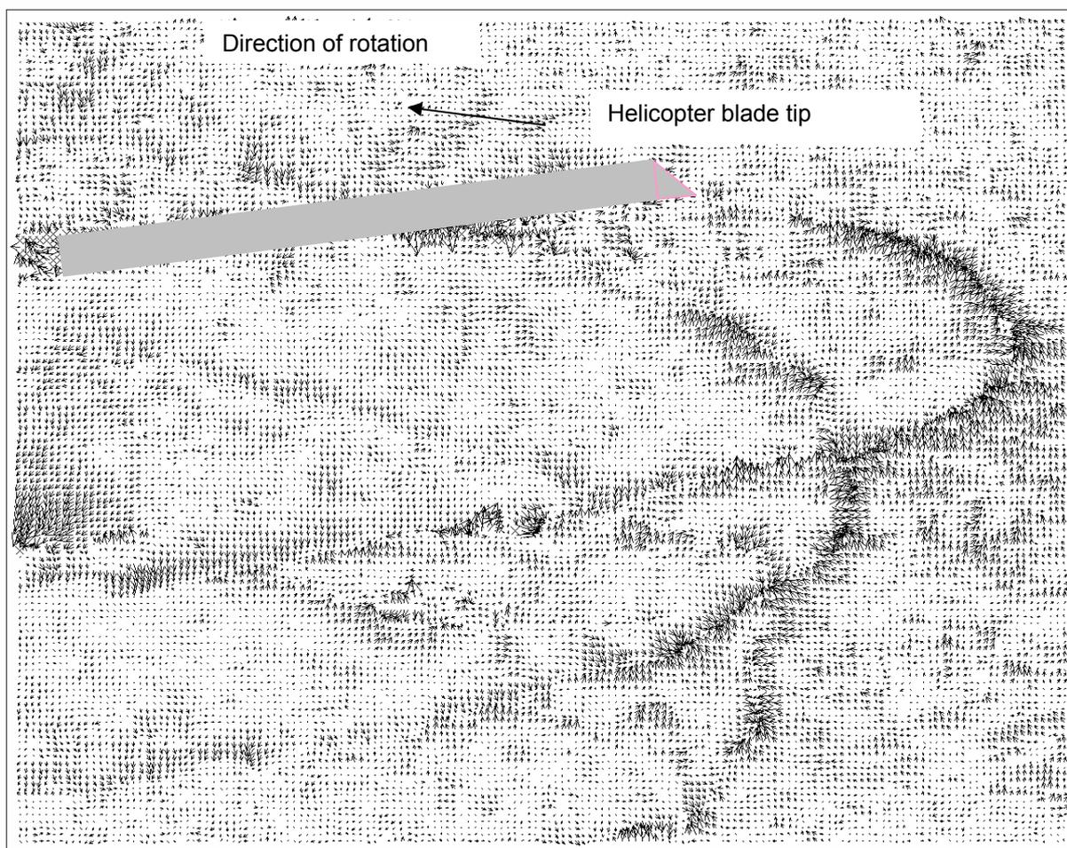
**Figure 7:** Vortex filaments. It can be seen that the vortex is not appearing directly at the rotor tip, since the vortex has to roll up first.
