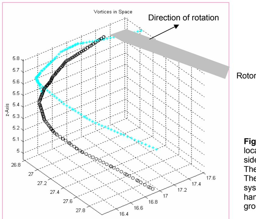
**Figure 8:** Result of the vortex localisation, viewed from the side. The dimensions are meters. The origin of the coordinate system is located at the right hangar edge on the apron ground.
