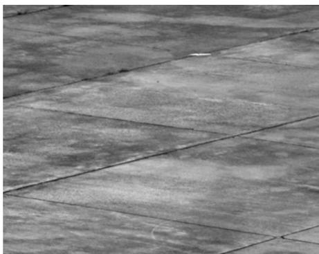
**Figure 6:** Background I imaged by camera I. This image was used as a reference for the cross-correlation of one test.
