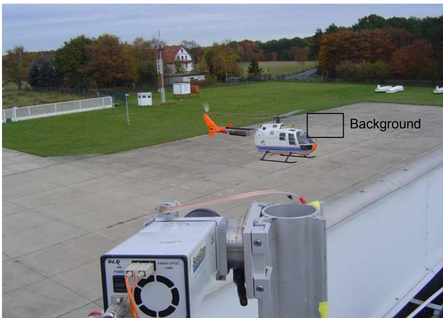
**Figure 5:** View from camera I over the helicopter towards background I, while the helicopter is hovering with its rotors into the investigation volume
