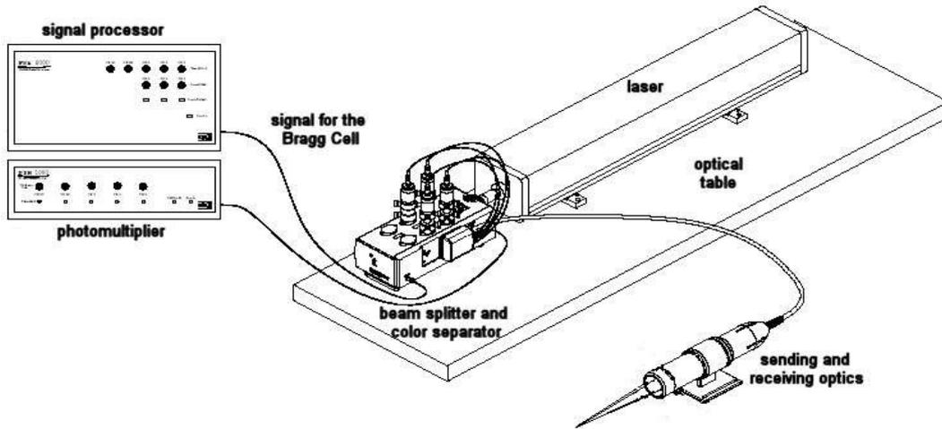
Figure 1: Optical components of the laser Doppler system
