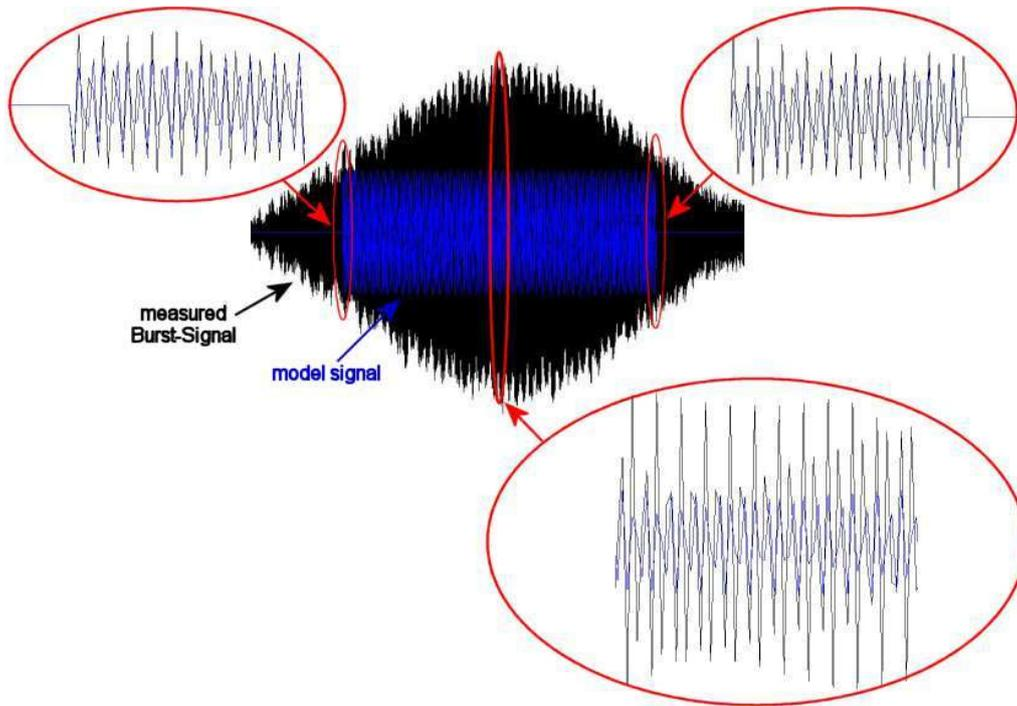
**Figure 7: Comparison between the measured and the model signal**
