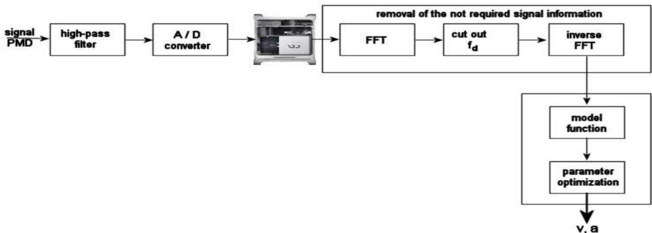
Figure 6: Flowchart of the signal processing
