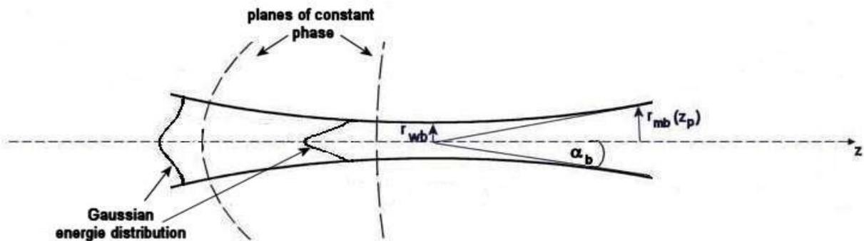
Figure 2: Gaussian laser beam
