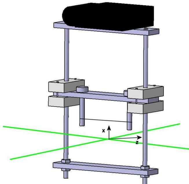
**Figure 8: Setup of the falling wire experiment**
