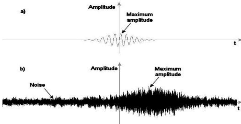
Figure 5: Simulated and measured burst signals
