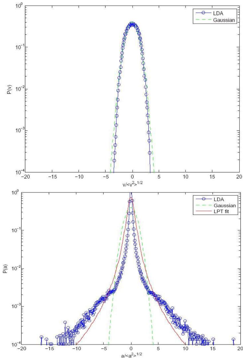
**Figure 13: PDFs from turbulence generator measurement**
