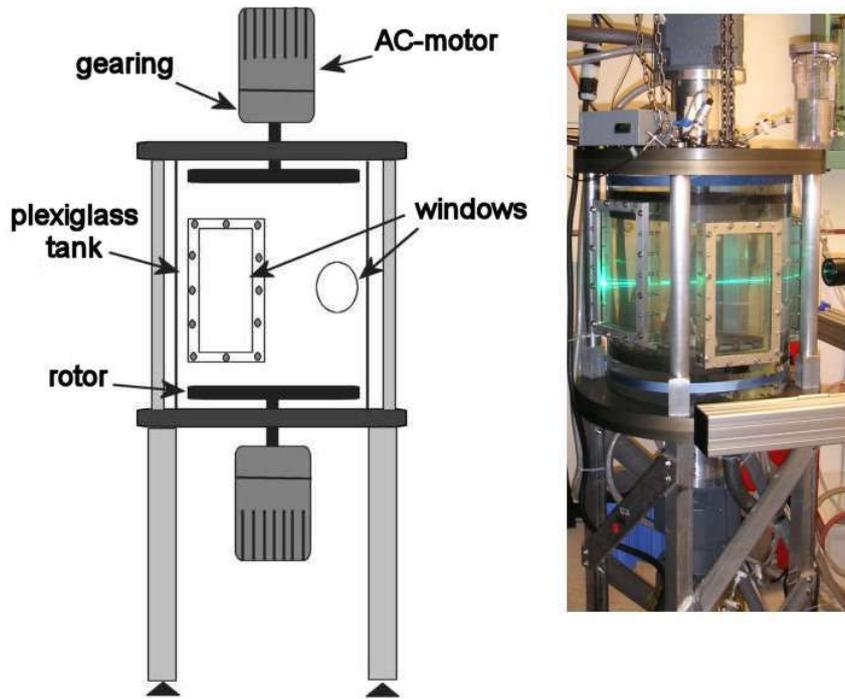
**Figure 11: Turbulence generator (French washing machine)**
