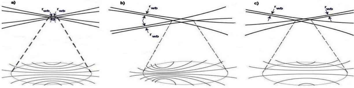
**Figure 3: Fringe divergence in the measurement volume**
