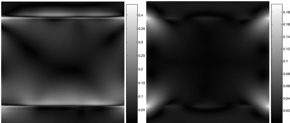
**Fig. 7. Left: RMS error ( $f$  is penalized everywhere), mean = 0.0734 px. Right: RMS error (no penalization of  $f$  on the interfaces), mean = 0.0212 px.**
