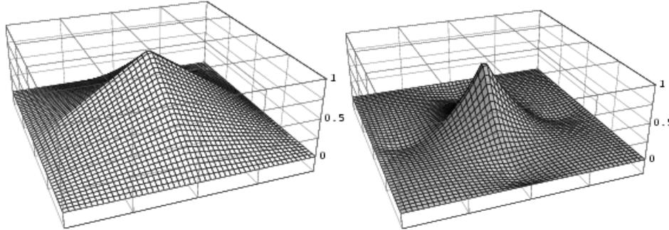
**Fig. 2. Left: Basis function  $\phi$  of a bilinear finite element. Right: Basis function  $\psi$  of a biquadratic finite element.**
