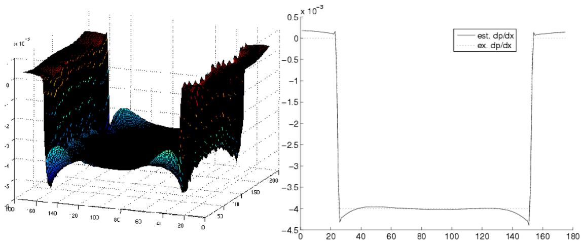
**Fig. 8. Left: Derivative of the pressure field in flow direction. Right: Profile of the averaged pressure derivative.**
