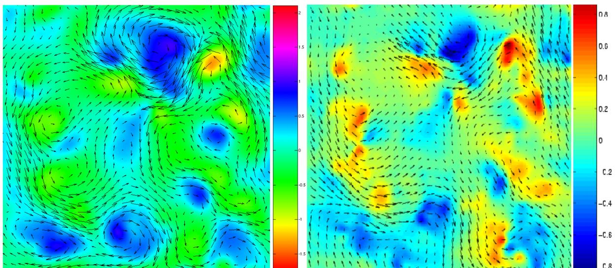
Fig. 10. Left: Resulting velocity field of control approach and its curl. Right: Resulting velocity field of Horn&Schunck approach and its curl.
