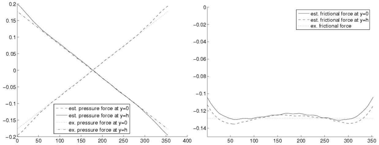
**Fig. 6. Left: Pressure-induced force at  $y = 0$  and  $y = h$  (estimated vs. exact). Right: Frictional force at  $y = 0$  and  $y = h$  (estimated vs. exact).**
