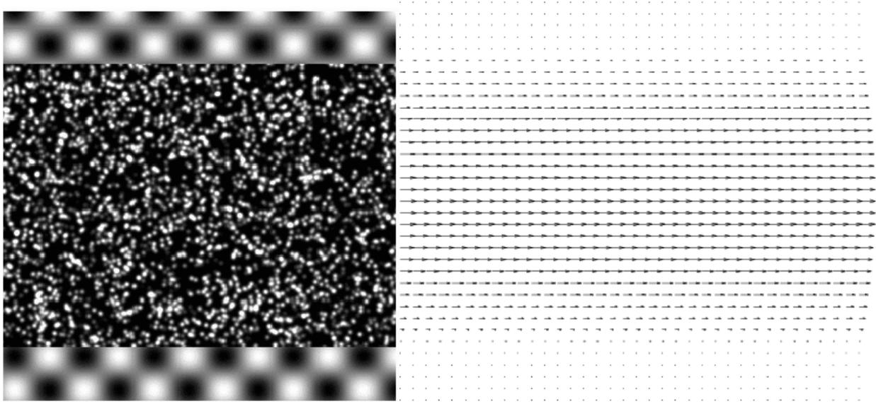
Fig. 3. Left: Synthetic PIV image. Right: Poiseuille velocity field.
