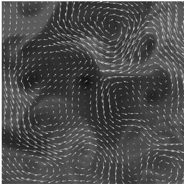
Fig. 9. Real image and its incompressible 2D flow field.
