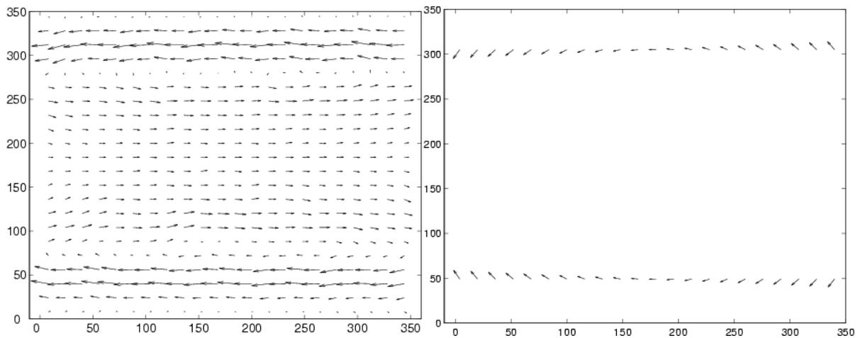
Fig. 5. Reconstructed body force. Note that the arrows are scaled in order to be visible. Left:  $f$  is penalized everywhere (scaling factor: 2000). Right: no penalization of  $f$  at the interfaces (scaling factor: 50).
