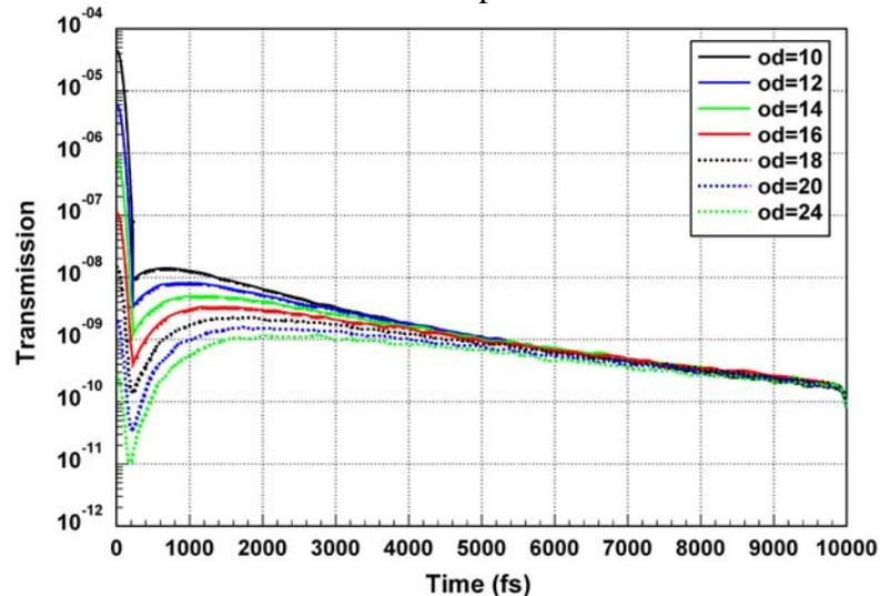
Fig. 11 Transmitted light (in log scale) versus time with optical depth as a parameter. The length of the cell is  $L=5\text{mm}$ , the particle diameter is  $d=1\ \mu\text{m}$ , particle refractive index is  $n=1.58-0.001i$ , absorption coefficient in water is  $K_T=1.5\ 10^{-4}\ \text{fs}^{-1}$  and the collection angle is  $\Delta\theta=0.07^\circ$
