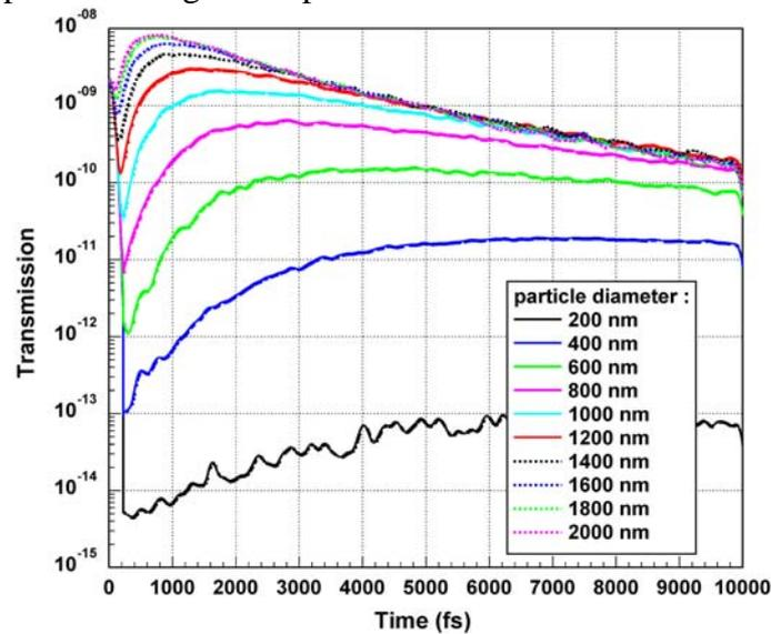
Fig. 12a Transmitted light versus time (in log scale) with the particle size as parameter and a constant optical depth. Other parameters are unchanged with respect to previous figures
