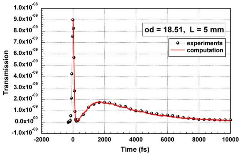
Fig. 5 Comparison between experiments and Monte Carlo simulation for a 5 mm cell. The optical depth  $od=18.51$  is measured from the experimental ballistic peak maximum. The particles diameter is  $d=1 \mu\text{m}$ . The absorption coefficient of water,  $K_T=1.5 \cdot 10^{-4} \text{ fs}^{-1}$  and the collection angle  $\Delta\theta=0.065^\circ$  correspond to the best fit values
