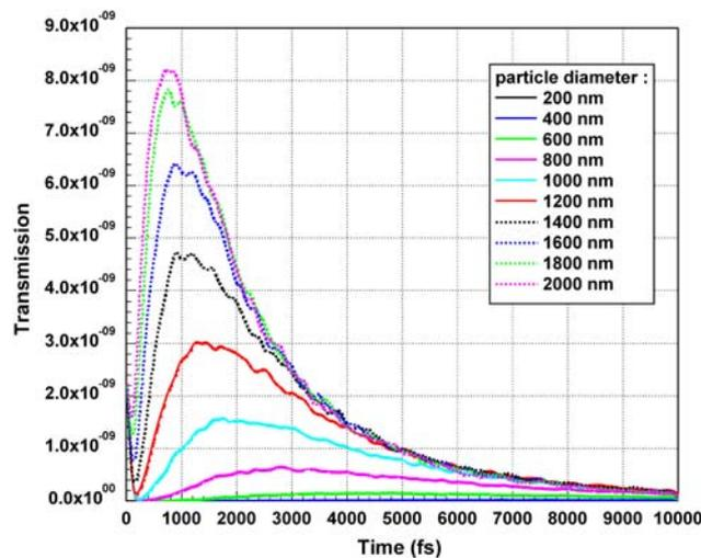
Fig. 12b Transmitted light versus time (in linear scale) with the particle size as parameter and a constant optical depth. Other parameters are unchanged with respect to previous figures
