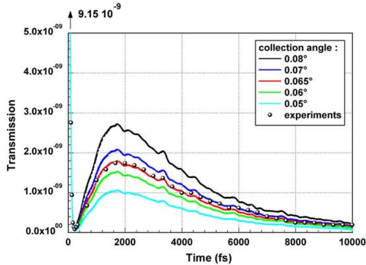
Fig. 6 Influence of collection angles  $\Delta\theta$ . Other parameters are unchanged with respect to figure 5
