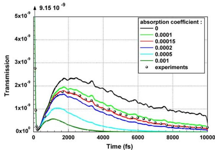
Fig. 7 Influence of the absorption coefficient  $K_T (\text{fs}^{-1})$ . Other parameters are unchanged with respect to figure 5
