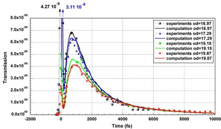
Fig. 9 Comparison between experiments and simulations for a 2 mm cell with various particles concentration. Other parameters are unchanged with respect to figures 5 and 8
