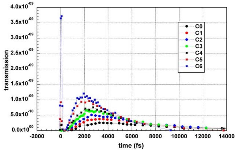
Fig. 3 Transmitted light versus time for decreasing polystyrene particle concentrations from C0 to C6. The cell length is  $L=5$  mm for all curves
