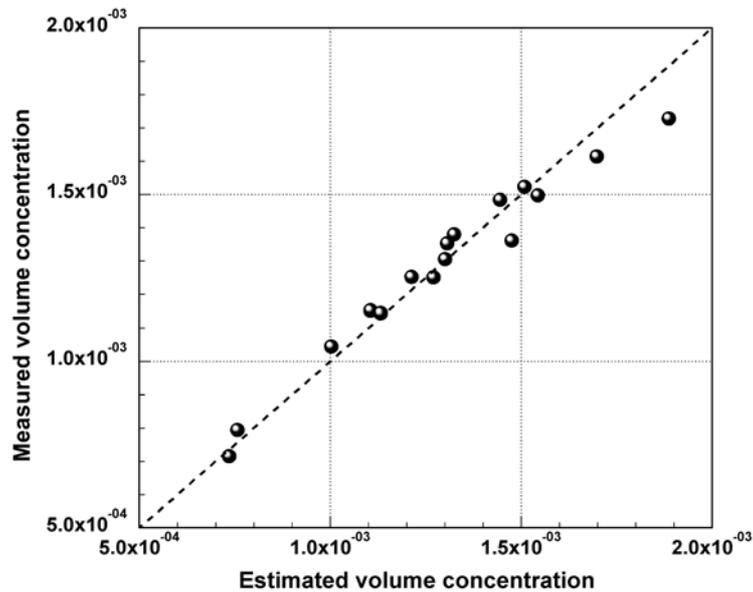
Fig. 4 Concentration measurements from ballistic peak intensities. The measured concentrations are compared with concentrations estimated from dilution processes
