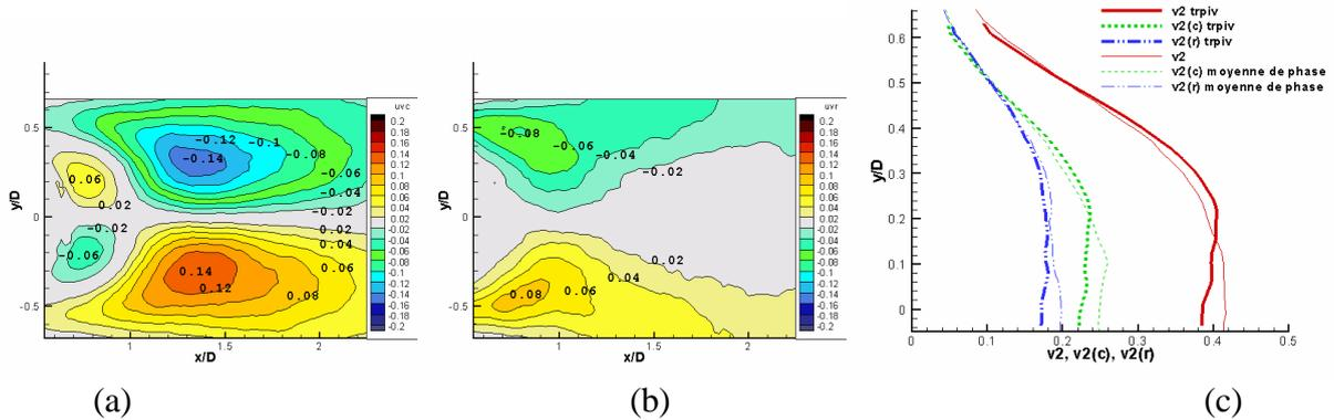
**Figure 10.** (a) and (b) Decomposition of the shear stress from phase averaging using POD coefficients. (c) Contributions of the organised and random fluctuations from phase averaging with POD coefficients compared with that evaluated from the spectra at  $x/D=1$  (legend as in Figure 6c)
