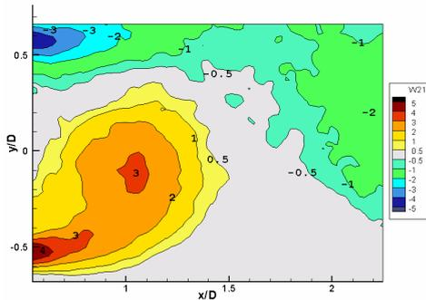
**Figure 8.**  $\langle \Omega_{21} \rangle$  component of the rotation rate tensor at  $f=\pi/4$  obtained by phase averaging using the POD coefficients
