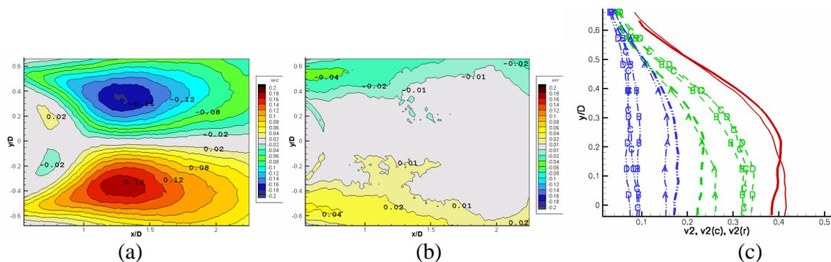
**Figure 7.** Decomposition of the Reynolds stresses by POD. (a) contribution of the 10<sup>th</sup> first mode to  $\overline{uv}$  (b) contribution of the rest of the modes; (c) decomposition of  $\overline{v^2}$  at  $x/D=1$  for different  $N$  compared with the organised and random contributions estimated from the spectra.
