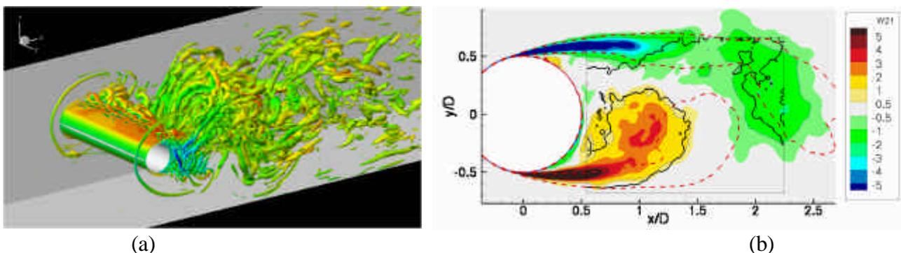
**Figure 11.** (a) Instantaneous visualisation of flow-field from DES with coarse time-step, (b) Comparison of phase-averaged isolines of  $\langle \Omega_{21} \rangle = \pm 1$  at  $f=p/4$  between DES with fine time-step (colours and feint blue line), DES with coarse time-step (red dashed line) and PIV (solid black line).
