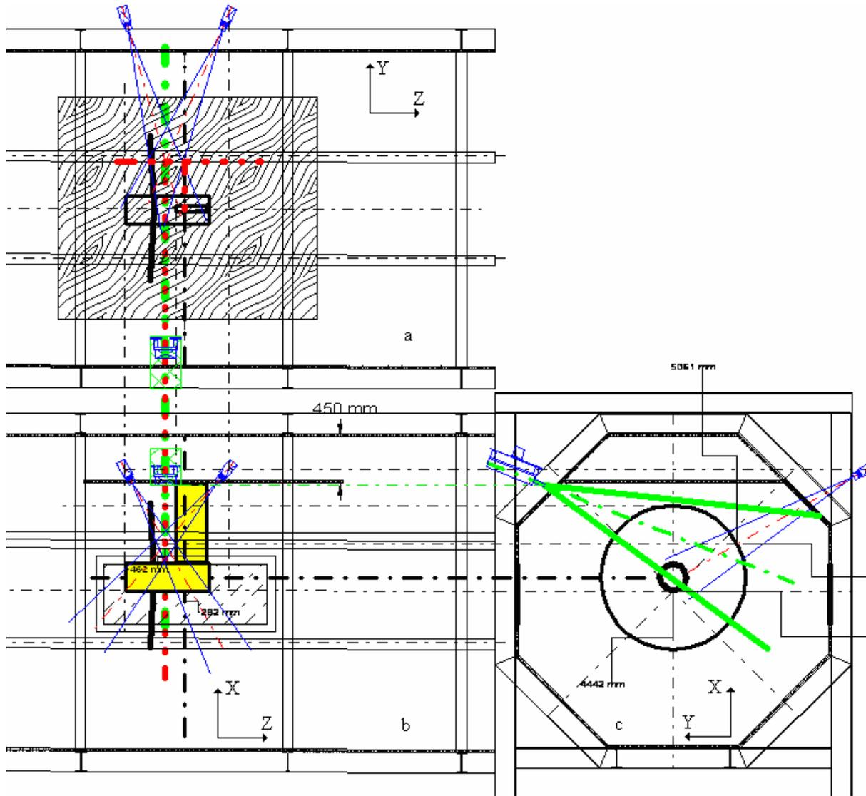
Fig.3. Schedule of PIV Set-up system
