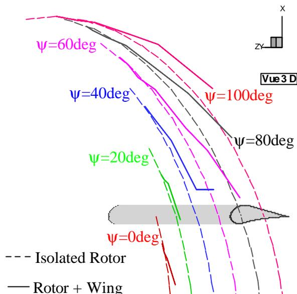
Fig.10. Tip paths in the isolated rotor wake (without wing, dotted lines) and in the cruise flight conditions (wing present, full lines):  $\mathbf{b}=0$  deg,  $\mathbf{q}=44$  deg,  $U_8=46\text{ms}^{-1}$ ,  $f=18.18\text{Hz}$ ,  $\mathbf{m}=0.575$
