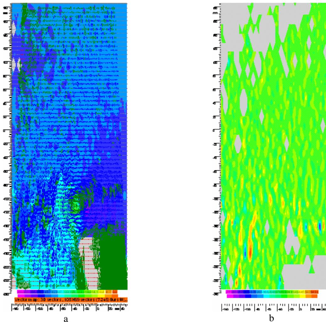
Fig.4. 3C View of the instantaneous flow behind the blade for a 2deg azimuth of the blade
