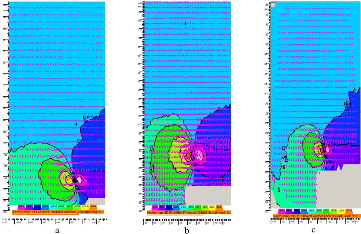
Fig.8. PIV measurements at plane  $Z/R=0$  behind the blade in cruise flight conditions ( $\mathbf{b}=0$  deg,  $\mathbf{q}=44$  deg,  $U_8=46\text{ms}^{-1}$ ,  $f=18.18\text{Hz}$ ,  $\mathbf{m}=0.575$ ) and for 3 blade azimuth positions
