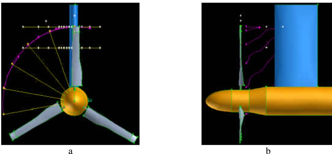
Fig.9. Blade tip vortex paths in cruise flight:  $\mathbf{b}=0$  deg,  $\mathbf{q}=44$  deg,  $U_8=46\text{ms}^{-1}$ ,  $f=18.18\text{Hz}$ ,  $\mathbf{m}=0.575$
