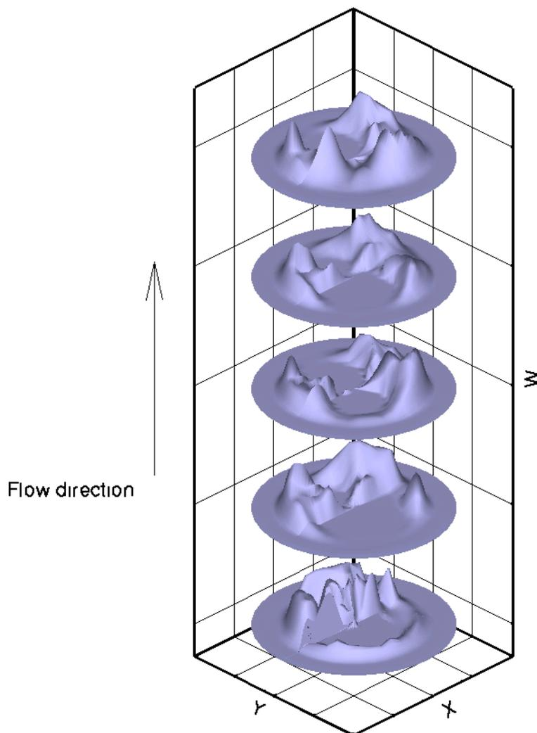
**Figure 7 Axial velocity at different heights of the tube filled with 30 mmspheres**
