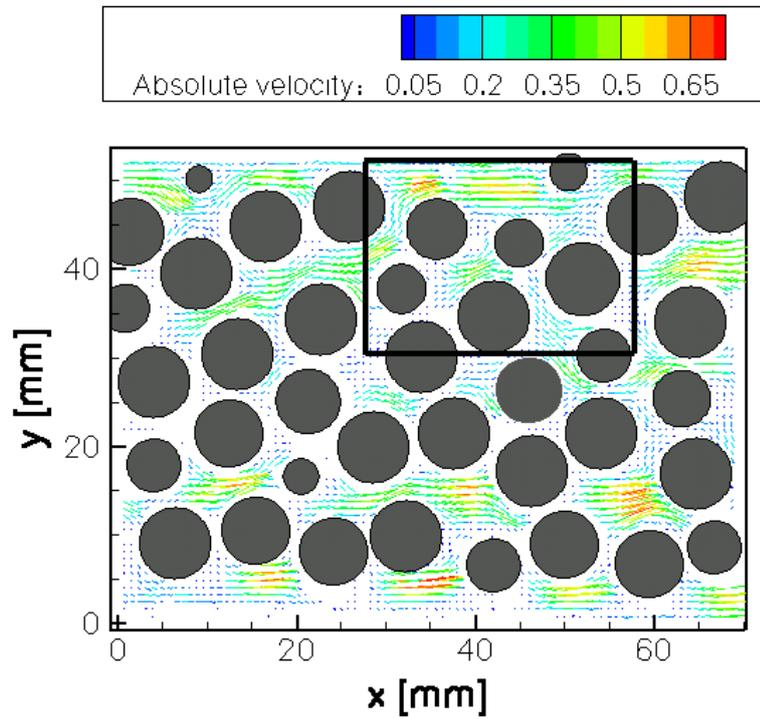
Figure 5: Velocity profile in the midplane of the tube filled with 9 mm spheres
