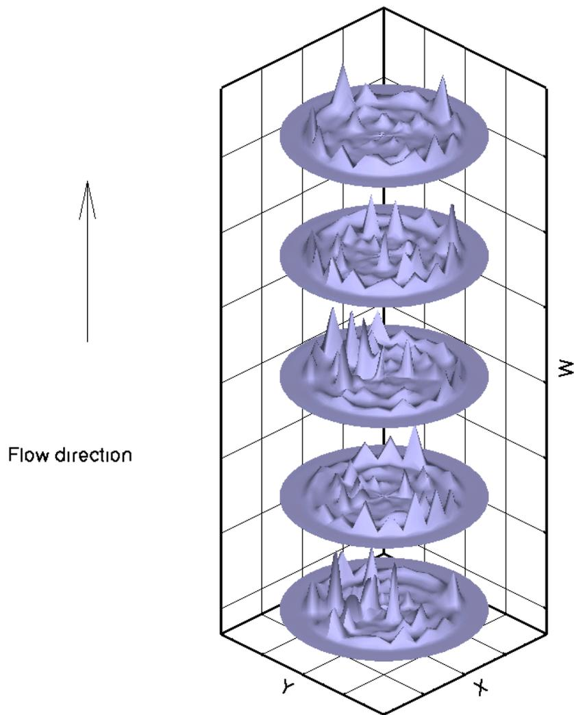
**Figure 9: Axial velocity at different heights of the tube filled with 9 mm spheres**
