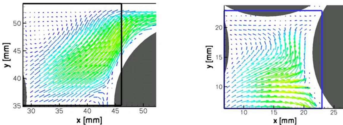
Figure 4: Details of the velocity profile in the midplane of the tube filled with 30 mm spheres.
