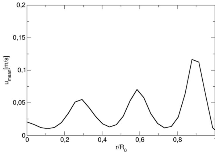
Figure 10: Mean axial velocity in the tube filled with 9 mm spheres
