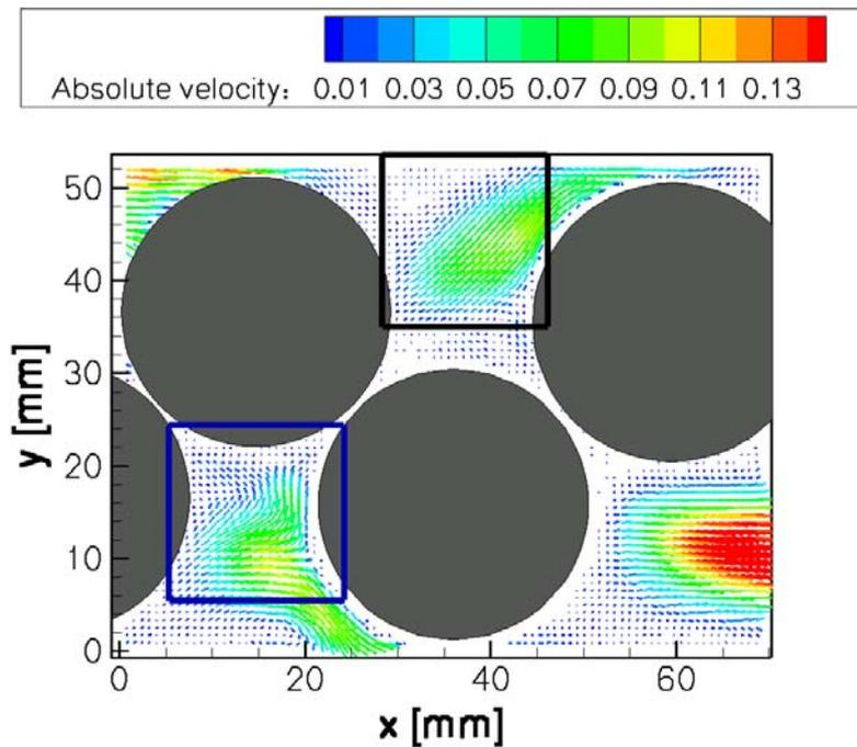
Figure 3: Velocity profile in the midplane of the tube filled with 30 mm spheres.
