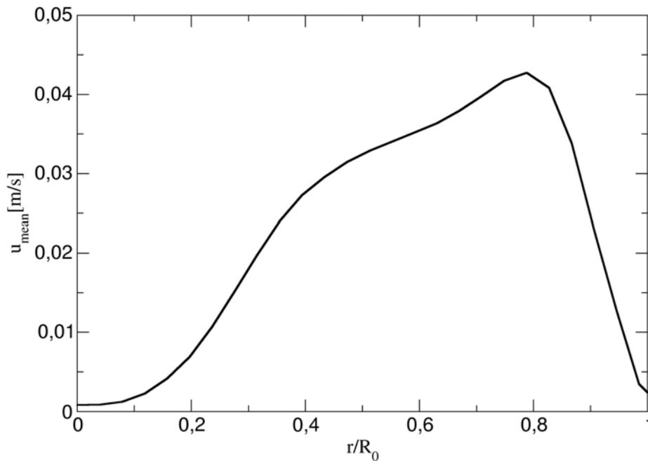
**Figure 8: Mean axial velocity in the tube filled with 30 mm spheres**
