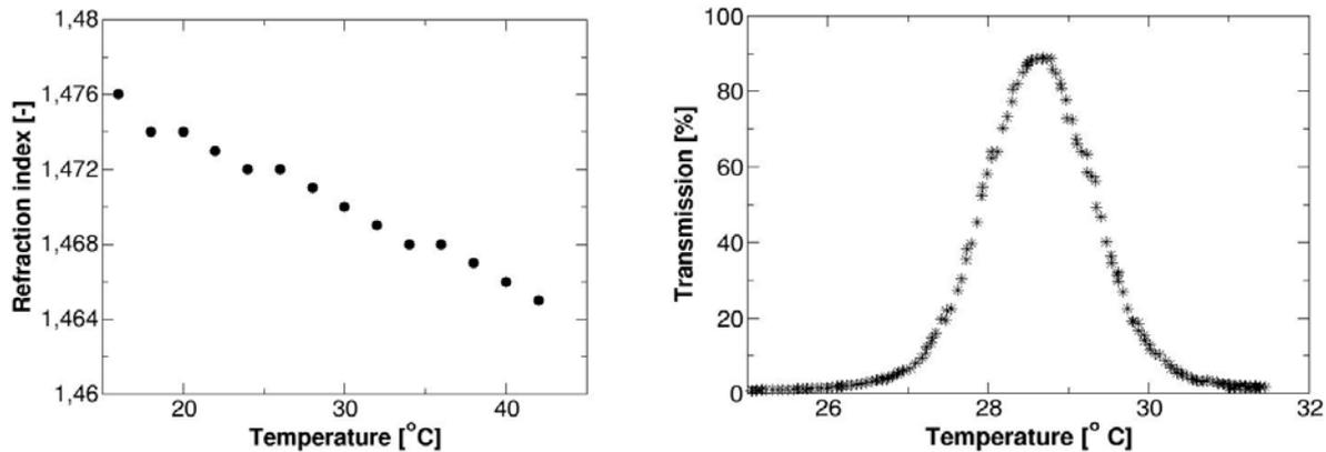
**Figure 2: Temperature dependence of the refraction index of oil (Shell Ondina 927), Optimal temperature for the accommodation of the refraction indexes.**
