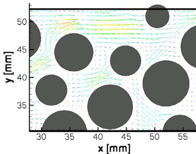
Figure 6 Detail of the velocity profile in the tube filled with 9 mm spheres
