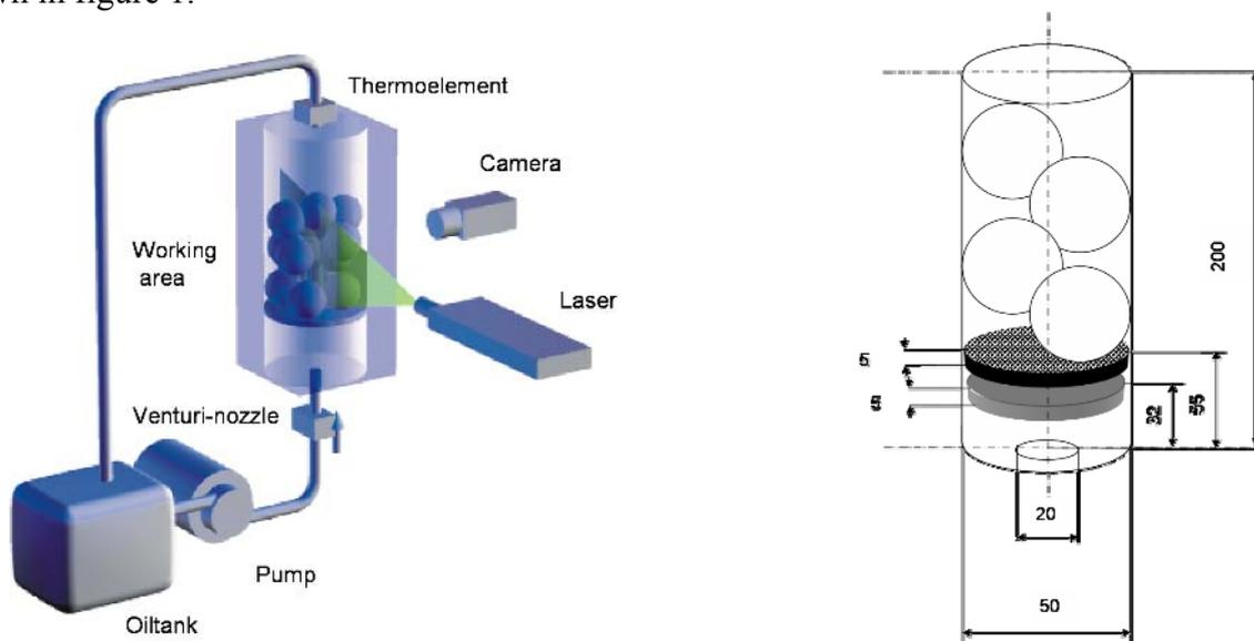
**Figure 1: Experimental setup and detail of the working area, dimensions in mm.**
