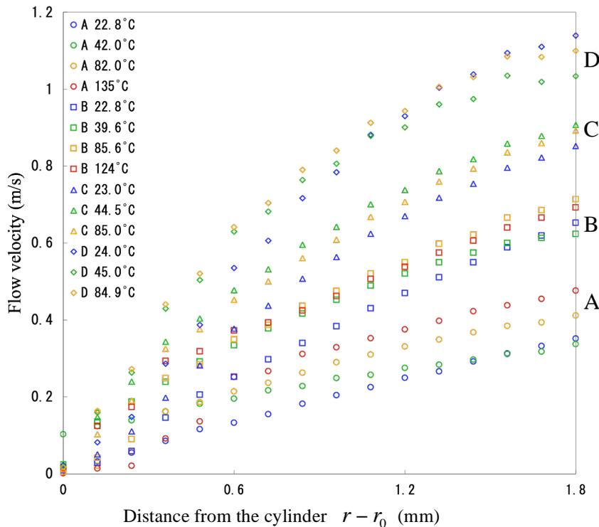
Figure 9: Velocity distribution of each condition near the cylinder surface. The horizontal axis and vertical axis are the distance from the cylinder surface and the flow velocity respectively.
