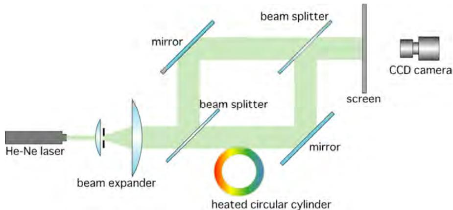
Figure 4: Mach-Zehnder interferometer.
