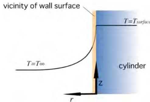
Figure 2: The temperature in the vicinity of cylinder surface.
