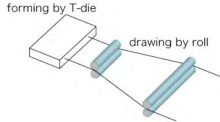
Figure 1b: T-die method. Molten polymer is formed by T-die and stretched by drawing roll.
