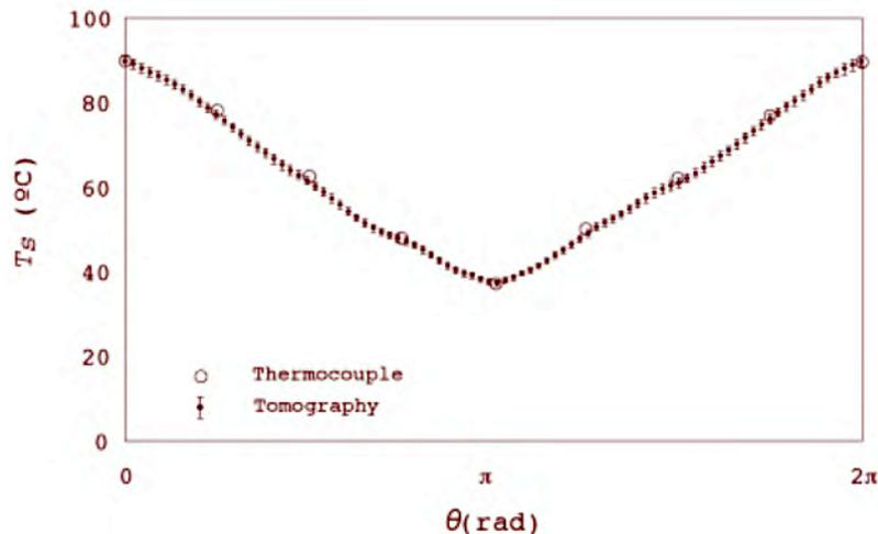
Figure 8: Comparison of measured surface temperatures by the method in first experiment and by the eight independent thermocouples fixed on the cylinder surface.
