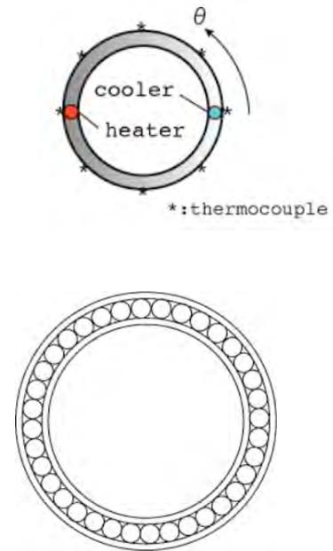
Figure 6b: Top view of the cylinder and the instrument, which makes forced convection around the cylinder used in the second experiment.
