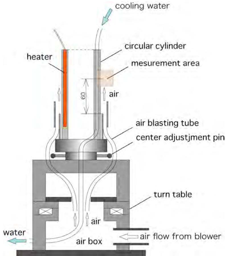
Figure 6a: An instrument makes forced convection around the cylinder.
