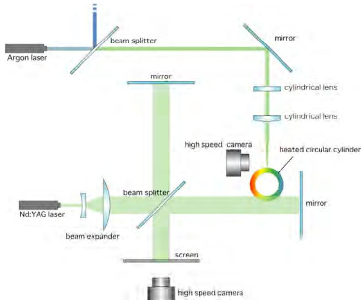
Figure 5: Second experimental setup using Michelson interferometer and PIV system. The air flow around the heated cylinder is forced convection.
