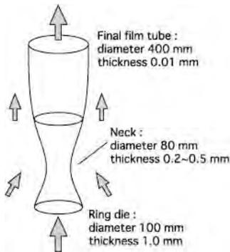
Figure 1a: Inflation method. Molten polymer blown out from ring die and is cooled by surrounding air jets simultaneously
