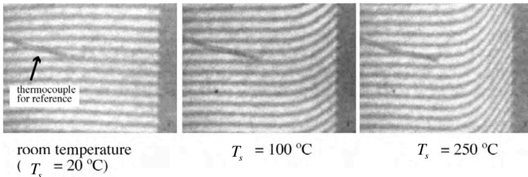
Figure 3: Captured finite fringe images at different surface temperatures. Ambient air temperature,  $T_\infty$ , was equal to  $20^\circ\text{C}$ . An inclined shaded line in the images is a thermocouple for the reference temperature measurement.
