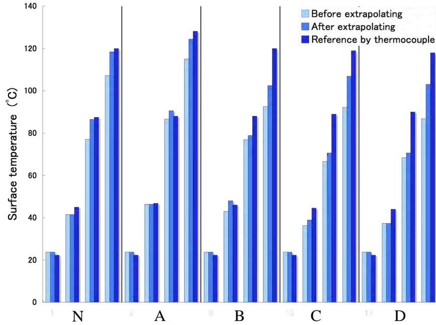
Figure 10: The temperature comparison among the temperature that was estimated by the method, the reference temperature captured by thermocouple, and the extrapolated temperature in different flow rates respectively. N means the condition that the blasting velocity is 0 m/s.
