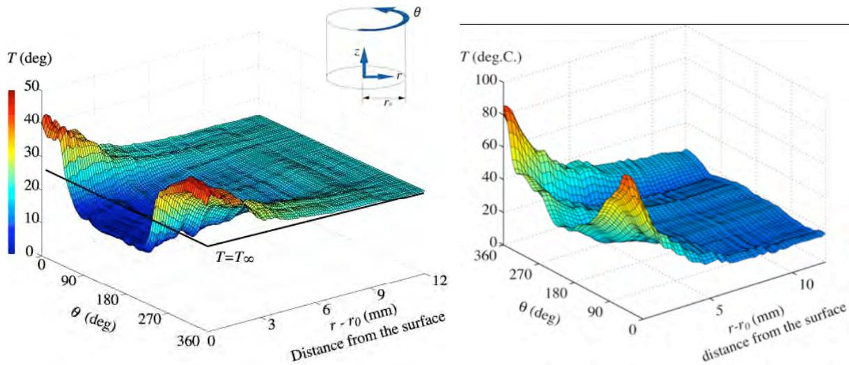
Figure 7a: The temperature distribution around the cylinder obtained by the first experiment. The highest temperature is 40 degrees and the lowest temperature is 15.6 degrees. Figure 7b: the highest temperature is 85 degrees and the lowest temperature is 20 degrees.
