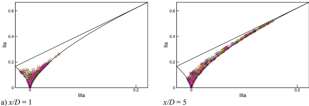
**Figure 12: States of turbulence in the wake of the co-rotating propellers pod drive model (color identification is the same as in figure 7)**
