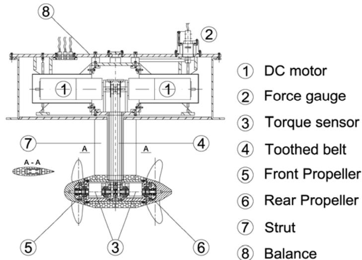
**Figure 3: Pod drive model and water tunnel balance**
