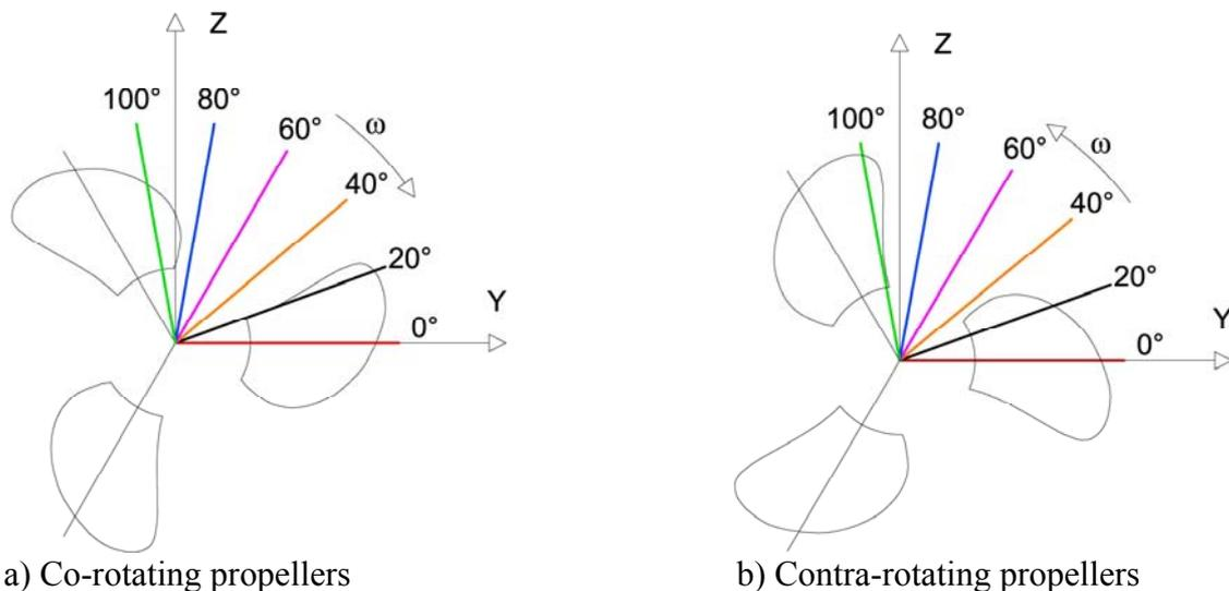
Figure 7: Position of radial profiles in the blade-fixed frame of reference
