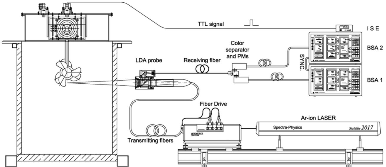
Figure 4: Experimental setup showing pod drive model in the water tunnel and the LDA system
