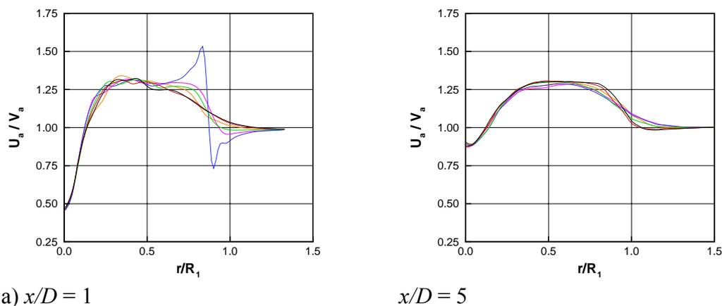
Figure 8: Axial velocity distribution in the wake of a co-rotating propellers pod drive model
