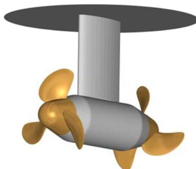
**Figure 1: Contra-rotating propellers pod drive model**
