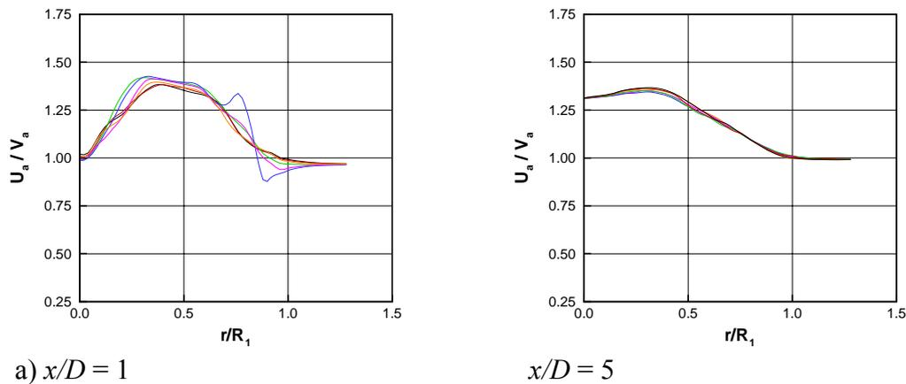
**Figure 10: Axial velocity distribution in the wake of a contra-rotating propellers pod drive model**
