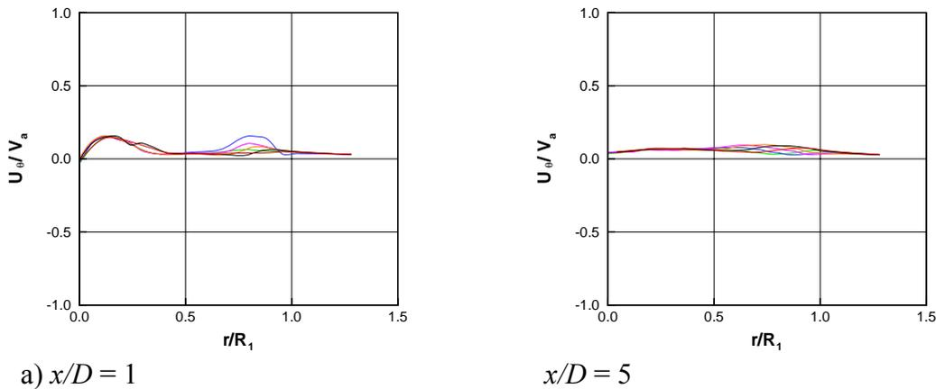
**Figure 11: Tangential velocity distribution in the wake of a contra-rotating propellers pod drive model**
