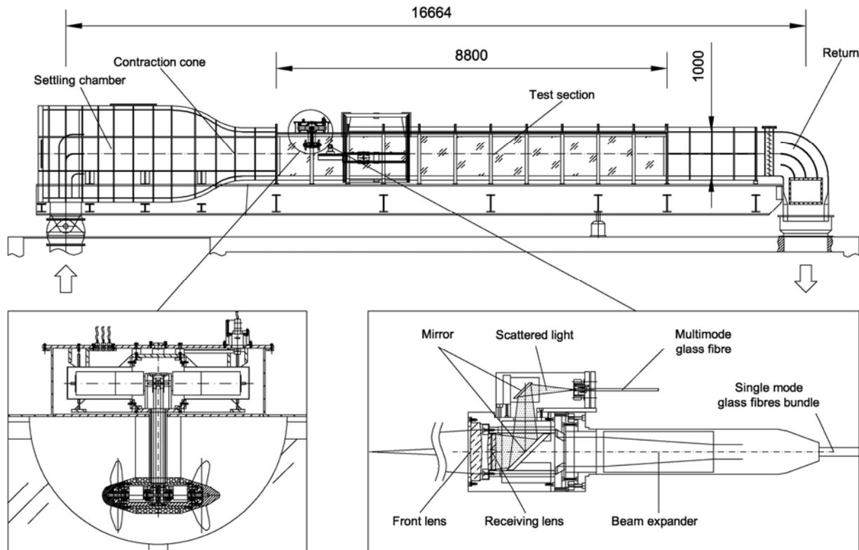
Figure 2: Water tunnel with ship propulsion test facility
