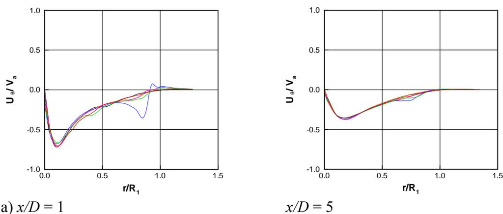
Figure 9: Tangential velocity distribution in the wake of a co-rotating propellers pod drive model
