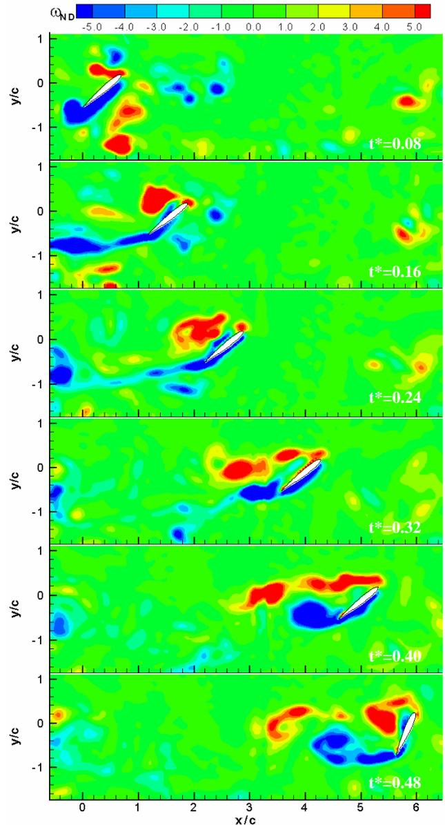
Fig. 2 Instantaneous non-dimensional vorticity contours from PIV measurements
