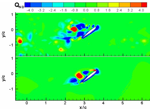
Fig. 1 Instantaneous non-dimensional  $Q$  contours at  $t^*=0.28$  from PIV measurements (top) and DNS results (bottom)
