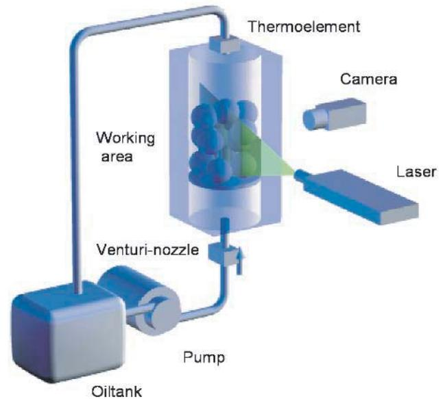
**Fig. 1** Experimental setup
