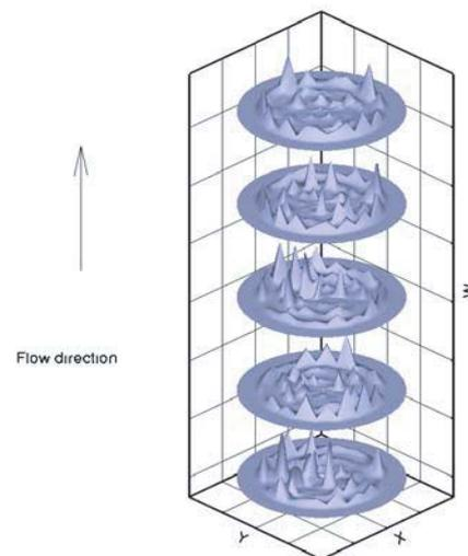
**Fig. 2** Axial velocity along the tube (9 mm spheres)
