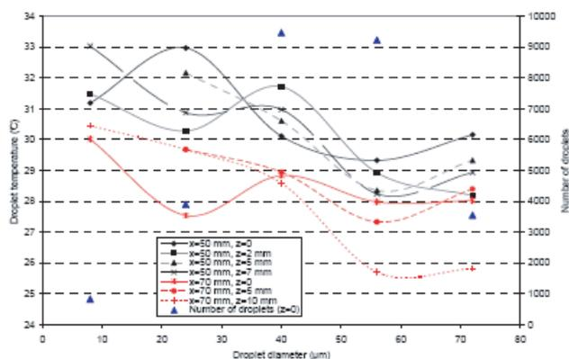
Fig. 1: Evolution of the droplet temperature as a function of the droplet diameter for different radial positions. The number of droplets used in the averaging process is also indicated.
