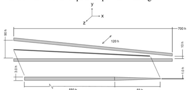
**Fig. 2** Dimensions of the flow channel and the splitter plate.
