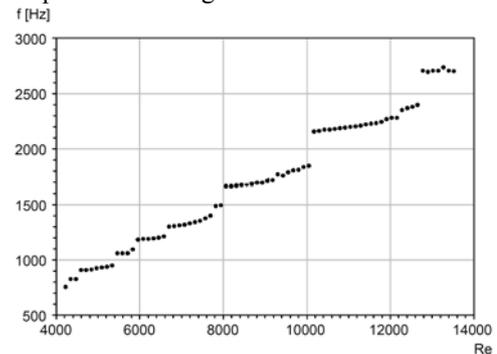
**Fig. 1** Vibration frequency of the plate tip as a function of Reynolds number.
