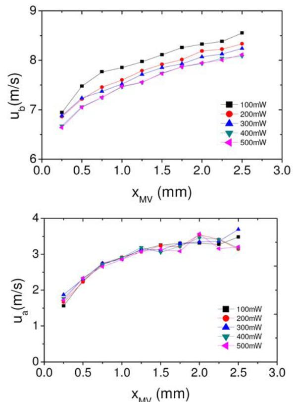
**Fig. 1** Before impact velocity (a) and after impact velocity (b) as a function of measurement volume height above the rigid wall. The different lines represent different laser power.
