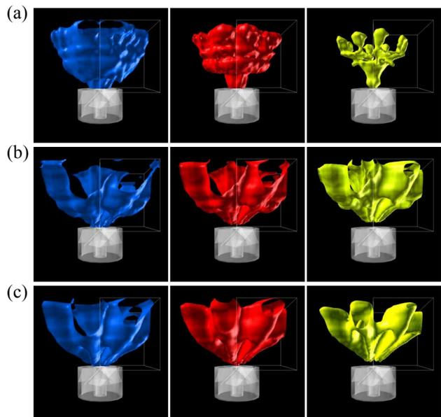
**Fig. 1** Three-dimensional distribution of probability of flame front existence (30% in unburnt side, 50% and 30% in burnt side from the left) for the no control case (a), continuous secondary fuel injection case (b) and intermittent secondary fuel injection case at 40Hz (c).
