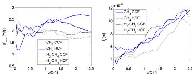
**Fig. 2:**  $u'_{rms}$  and  $l_t$  distribution averaged over  $r$ , plotted in axial direction.
