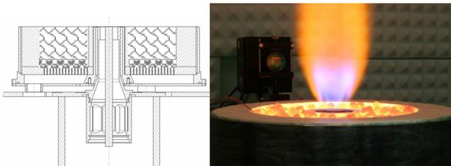
**Fig. 1:** Sketch of the TD1 swirl burner enclosed by the porous burner (left). Both burners during operation (right)
