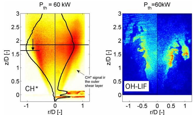
**Fig. 3:**  $CH^*$  chemiluminescence and OH-LIF distribution for cold (left parts) and hot (right parts) co-flow
