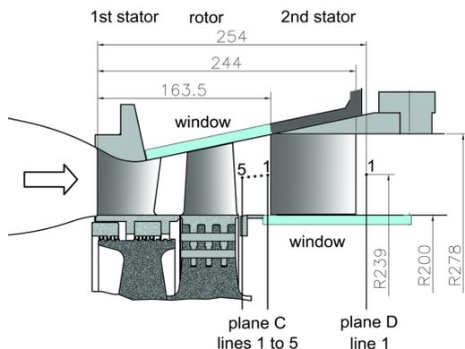
**Fig. 1:** meridional section of the transonic turbine (1½ stage), The dots indicate the measurement positions along five lines between the rotor and the 2<sup>nd</sup> stator and along one line behind the 2<sup>nd</sup> stator.
