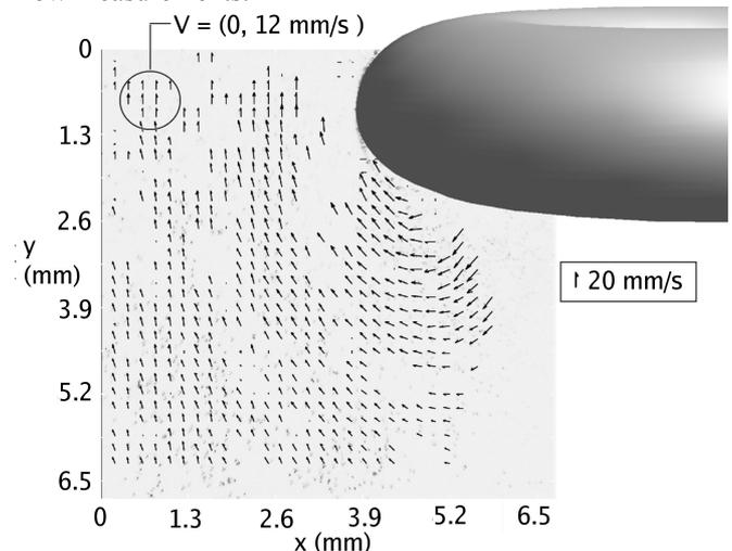
**Fig 2.** Velocity field near a downward traveling vortex ring. The drawn vortex ring is added for clarity.
