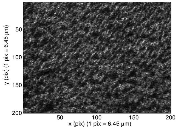
**Fig 1.** Holographic reconstruction of the hydrogen bubble field.
