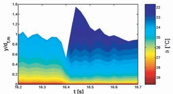
Fig. 2 Temperature distributions in a single wave.
