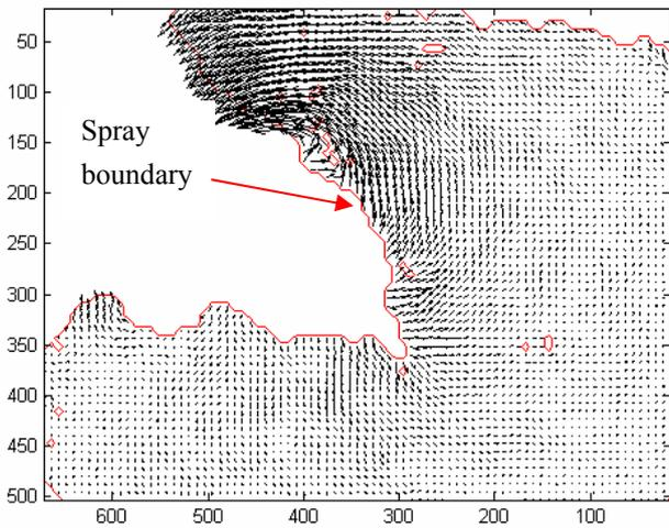
**Figure 1 : Two-phase flow filtered instantaneous velocity flow field.**
