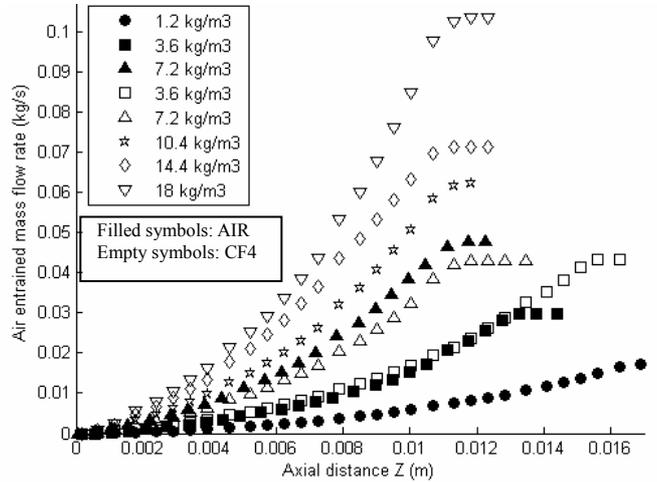
**Figure 2 : Cumulative air entrainment mass flow rate at various ambient density.**
