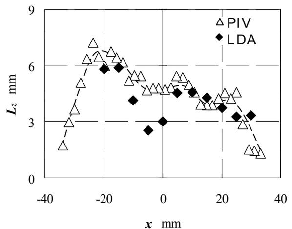
**Fig. 1** Comparison of the length scales by LDA with slotted correction method and PIV.
