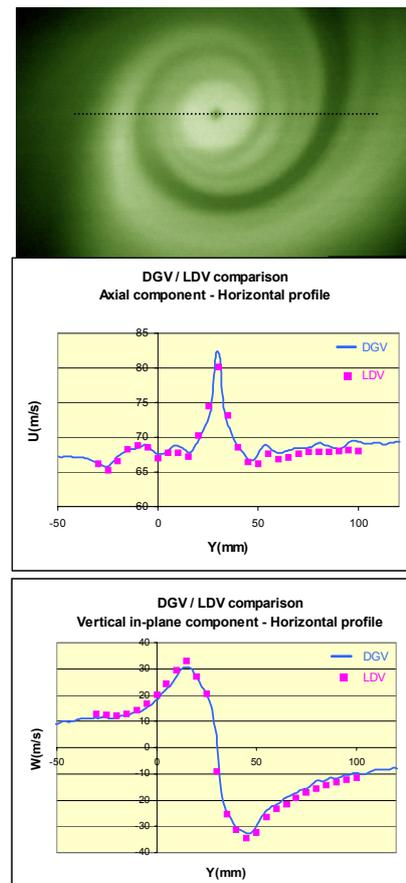
**Fig. 2** Tip vortex in the wake of a 2D airfoil in the ONERA F2 wind tunnel. Doppler map (top). Velocity profiles through the vortex: DGV/ LDV comparison
