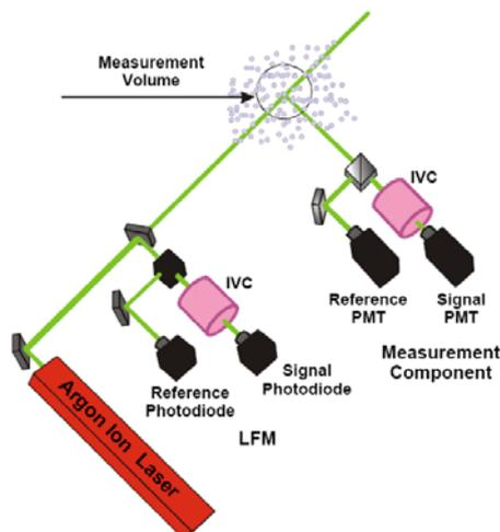
**Fig. 1** Schematic of the Point Doppler Velocimeter.
