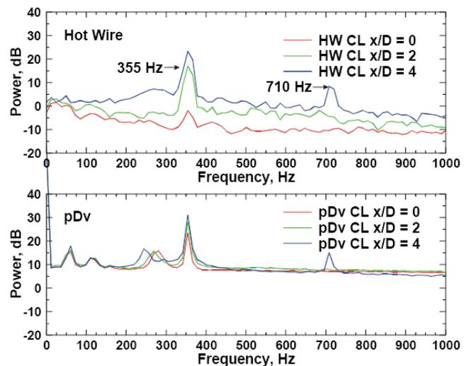
**Fig. 3** Spectral content of the flow exiting a two-inch pipe.
