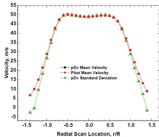
**Fig. 2** pDv and pitot probe velocity profiles obtained at the  $x/D = 2$  location of the 50.8-mm jet flow.
