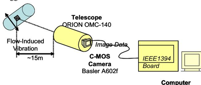
**Fig. 1** Super-Long Range PIV System for Non-Contacting Measurement of FIV
