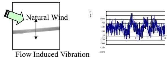
**Fig. 3** Time Domain Vibration of Transmission Line
