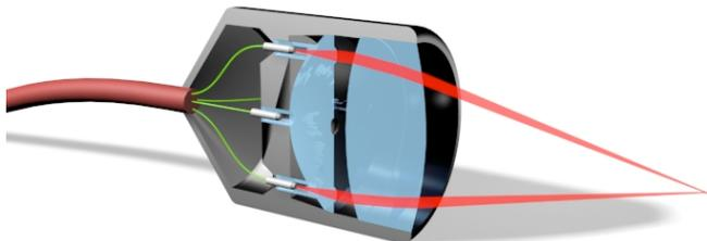
2d-LDV-measurement head with integrated optical element
