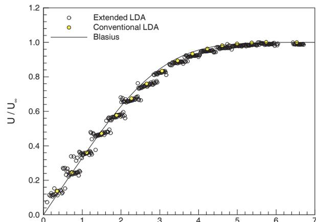
Figure 2: Averaged Velocity Profile of the Laminar Boundary Layer at  $x = 185$  mm
