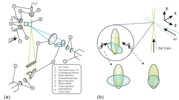
Figure 1: Schematic diagram of extended LDA-system
