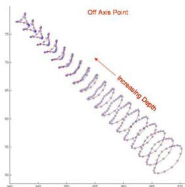
**Fig. 1.** Actual and model predicted paths of a single correspondence feature. The small circles represent actual image positions of the imaged feature at varying distances (depths) from an AWS camera focal position. The solid lines represent the calibration model's re-projected path.
