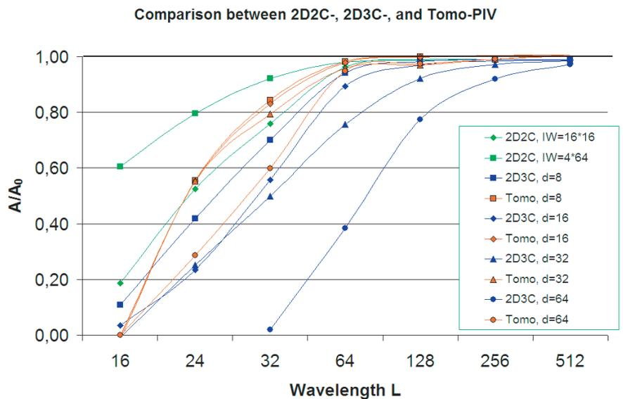
**Fig. 2.** Reduction in measured amplitude as a function of wavelength  $L$  and light sheet thickness  $d$  for 2D-PIV (green lines), Stereo-PIV (blue), and Tomo-PIV (red).
