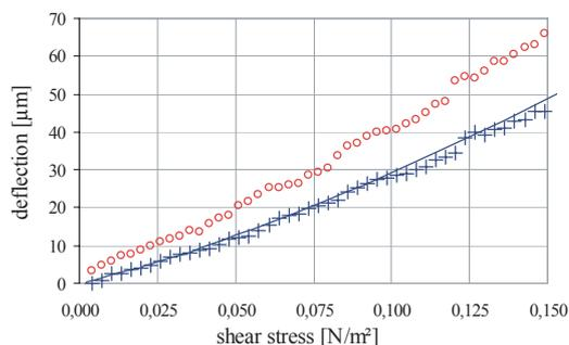
**Fig. 3** Comparison of theoretical and measured deflection. The rheometer speed was continuously increased. The fluid is water at 25°C. Solid line: theoretical pillar deflection, + measured pillar tip deflection, o: measured pillar plus bubble deflection
