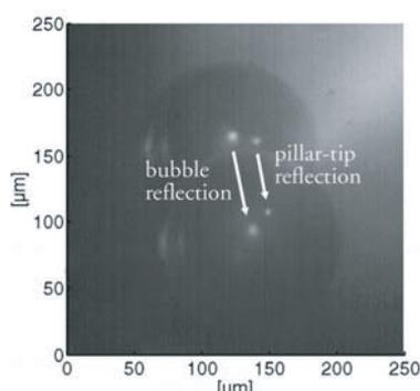
**Fig. 2** Comparison of the non-deflected and deflected bubble position and the reflections in detail. Arrows evidence the trajectories of the reflective spots.
