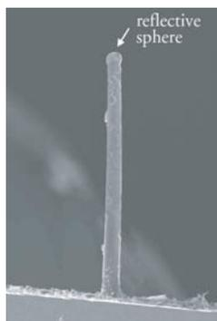
**Fig. 1** SEM of a single pillar sensor with reflective tip (height 470 $\mu\text{m}$ , diameter 25 $\mu\text{m}$ )
