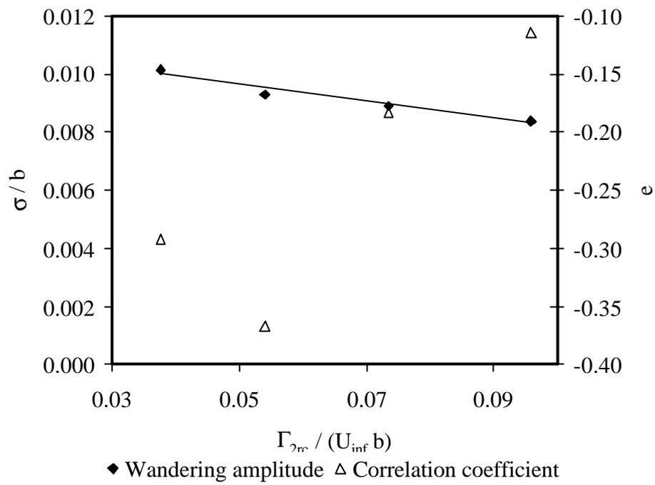
Figure 8. Variation of wandering amplitude and correlation coefficient with vortex strength.
