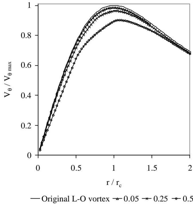
Figure 3. Mean tangential velocity profile extracted from re-centred data with varying grid spacing,  $\Delta/r_c$ .
