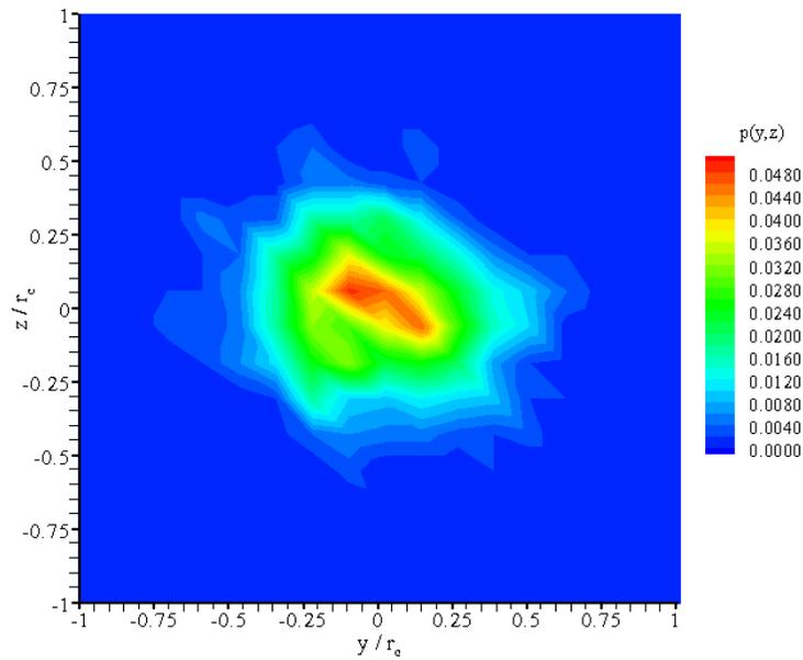
Figure 6. Probability density plot of vortex position for  $\alpha=8^\circ$  case at  $x/c=22.9$ .
