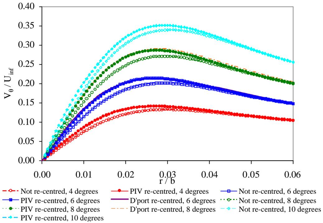
Figure 5. Radial profiles of tangential velocity for non re-centred and re-centred data using the PIV method and the Devenport method.
