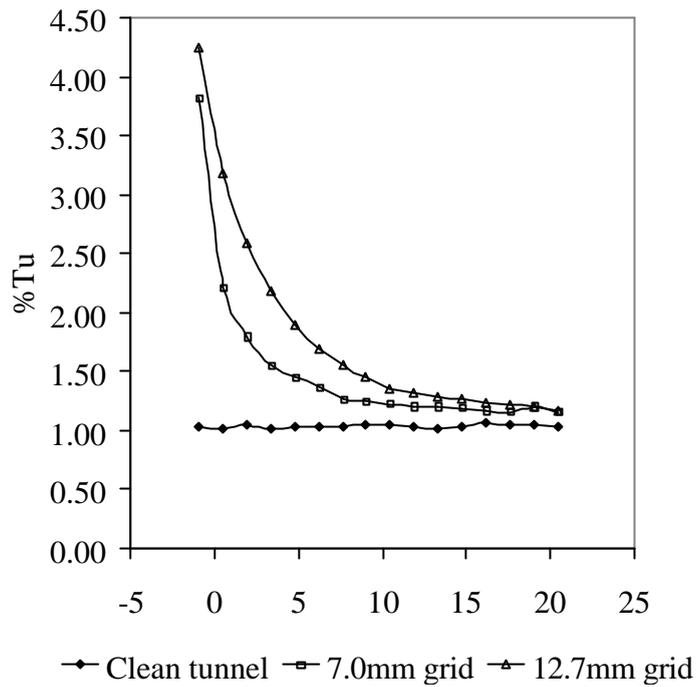
Figure 9. Variation of turbulence intensity with stream-wise distance.
