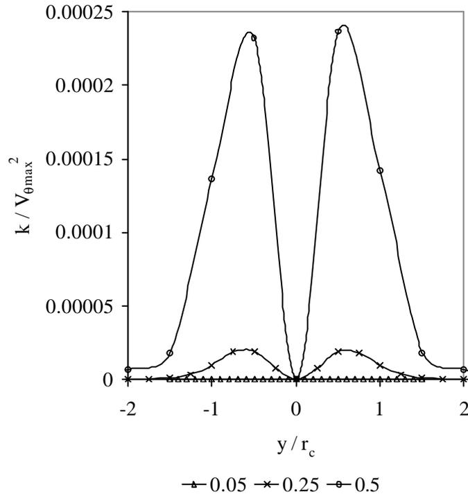
Figure 4. Cross-stream fluctuation energy after re-centring with varying grid spacing,  $\Delta/r_c$ .
