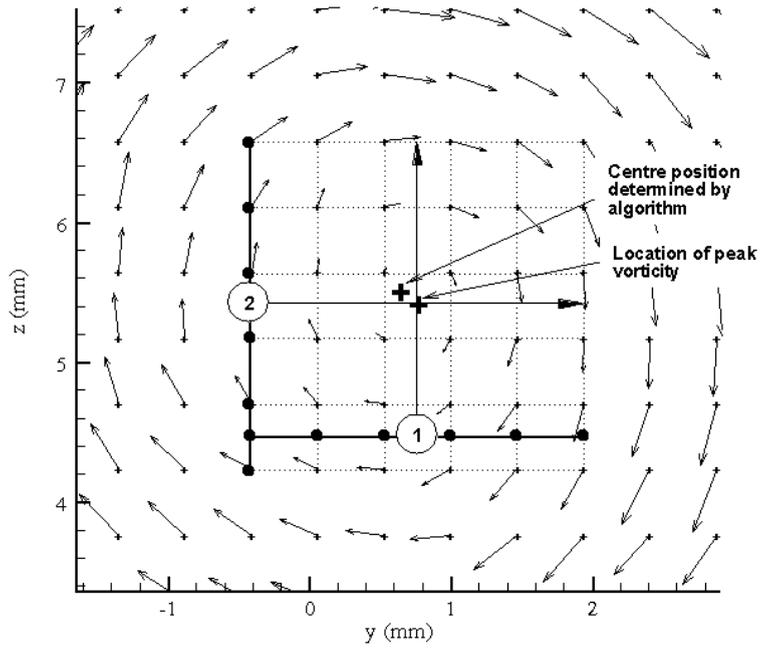
Figure 1. Diagram illustrating vortex centre finding algorithm.
