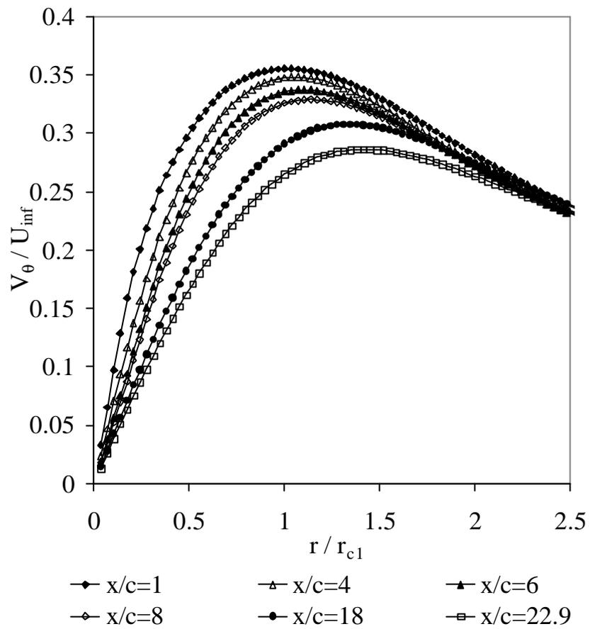
Figure 12. Radial profiles of tangential velocity for 70mm chord wing with stream-wise distance in the clean tunnel.
