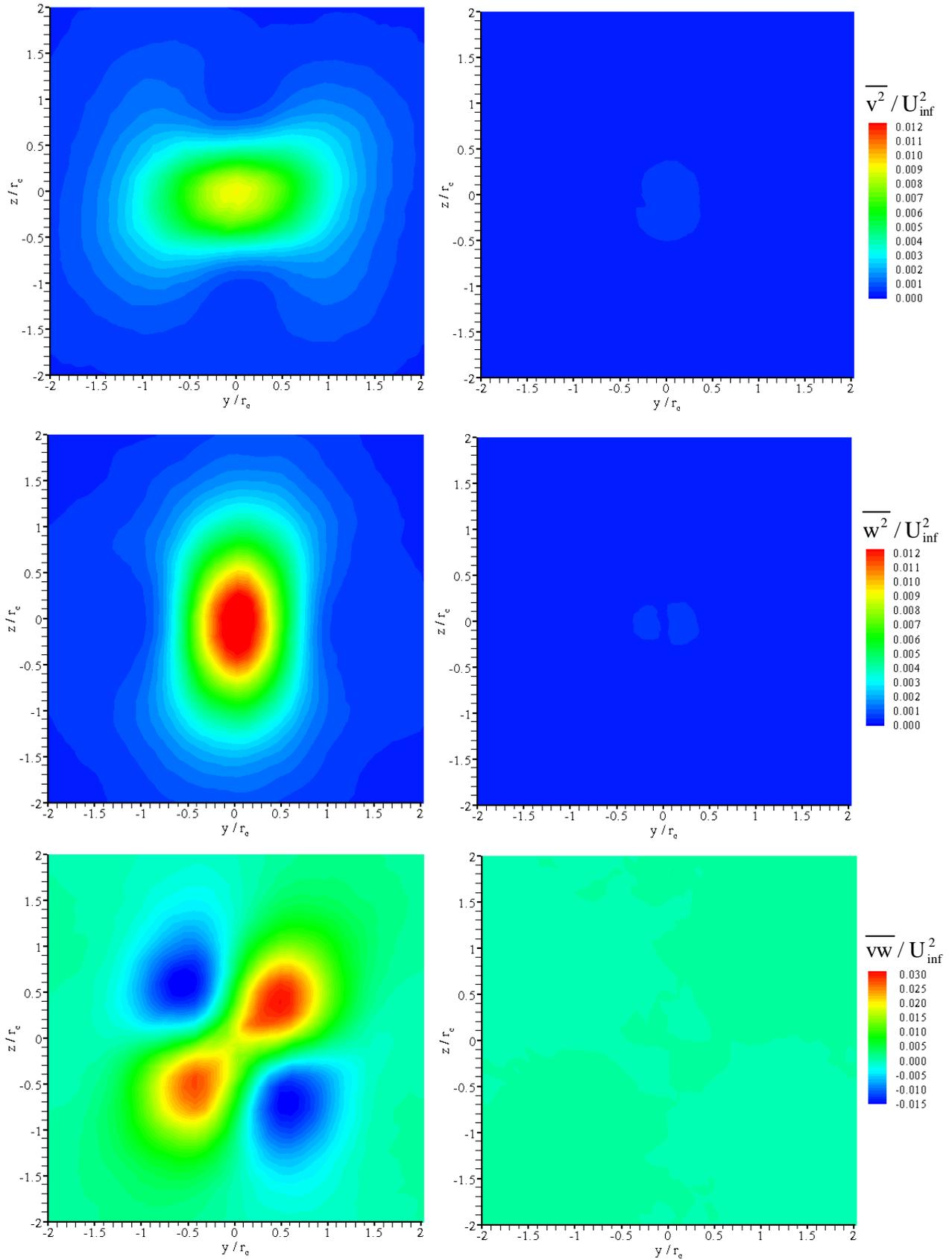
Figure 7. Reynolds stress components calculated from non re-centred data (left hand side) and re-centred data (right hand side).
