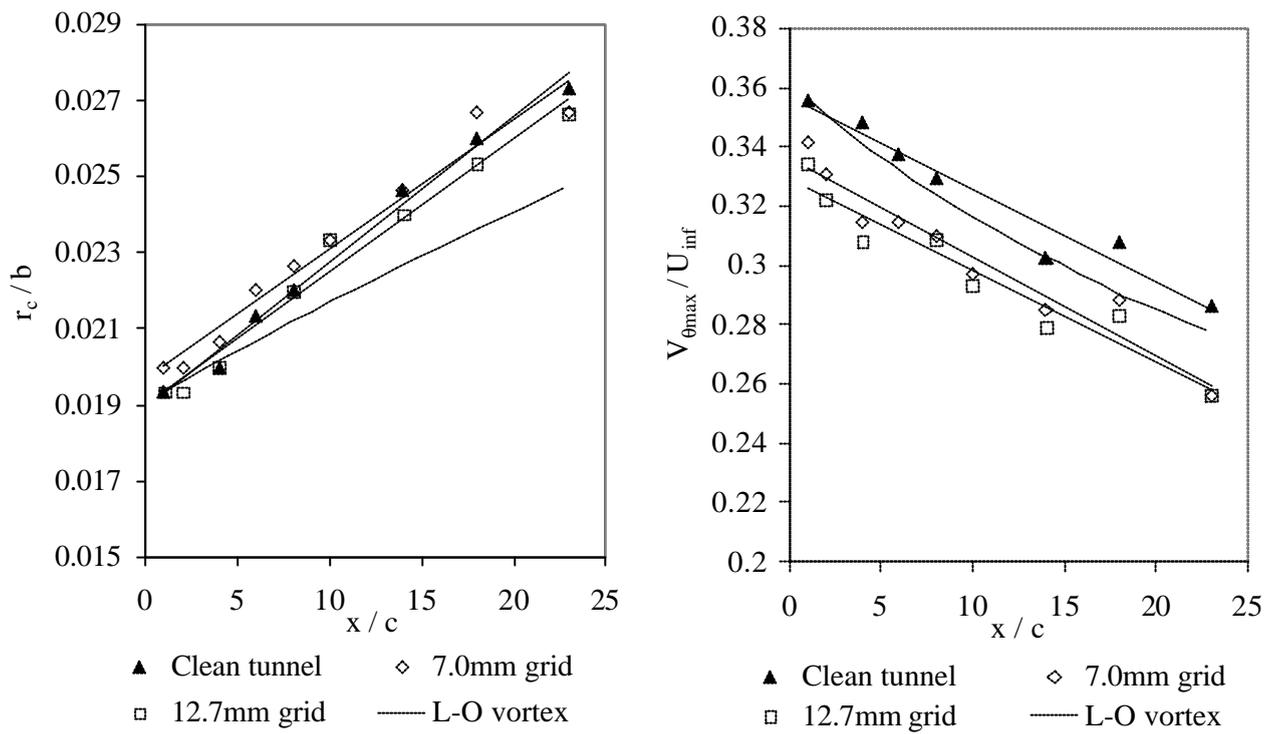
Figure 13. (a) Variation of core radius with stream-wise distance. (b) Variation of peak tangential velocity with stream-wise distance.
