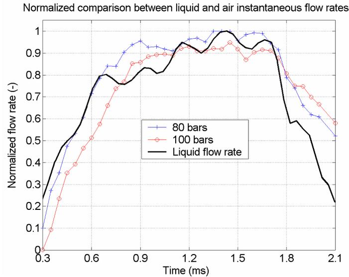
Figure 16 : Liquid and gaseous instantaneous flow rates
