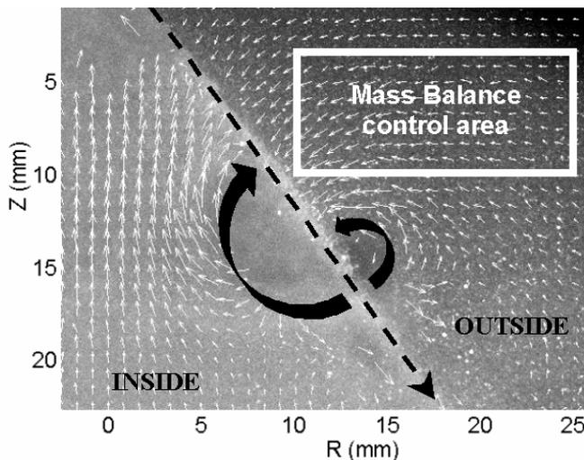
Figure 14 : Spray geometry and air motion (maximum velocity : 9m/s,  $P_{inj} = 50$  bars,  $p_w = 1$  ms)
