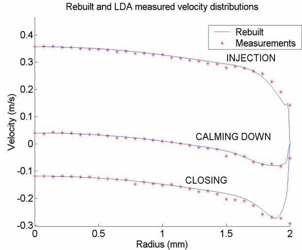
Figure 4 : Velocity distributions by LDV (\*) and rebuilding theory (solid line)
