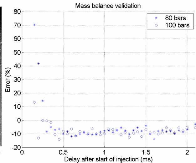
Figure 15 : Mass balance gap over an injection period
