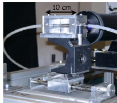
Figure 2 : Pyrex tube mounted on its 3D device
