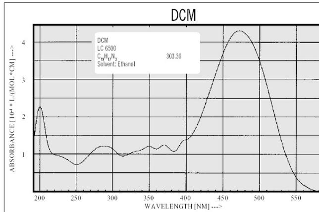
Figure 9 : Absorbance of a DCM-ethanol solution
