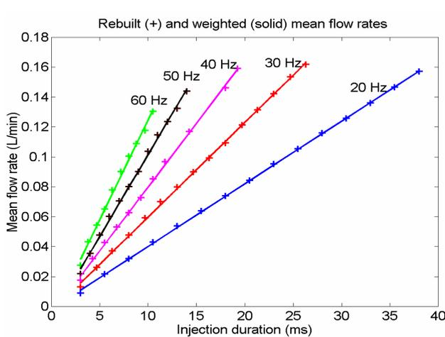
Figure 7 : Weighted (solid lines) and rebuilt (crosses) mean flow rates (various injection durations, frequencies)
