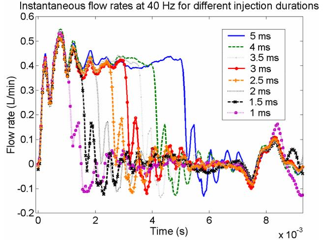
Figure 6 : Return of the opening pressure wave
