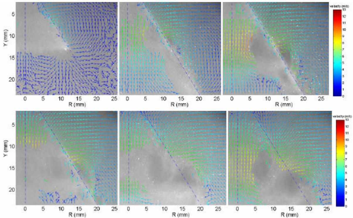
Figure 13 a, b, c, d, e, f : Air velocity fields by FPIV
