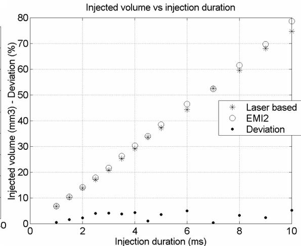
Figure 8 : Comparison between rebuilt (stars) and EMI2 (circles) injected volumes
