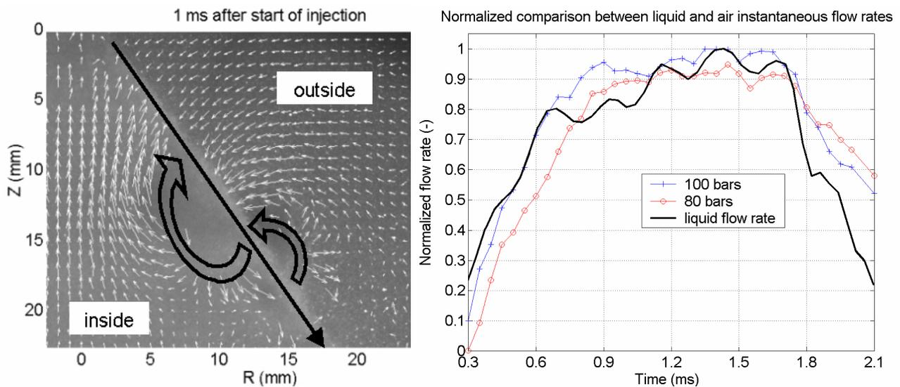
Fig. 1 : GDI injector transient analysis
