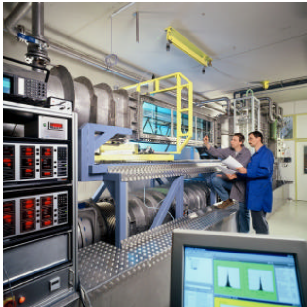
Fig.3: Matched Index Refraction tunnel at LSTM Erlangen
