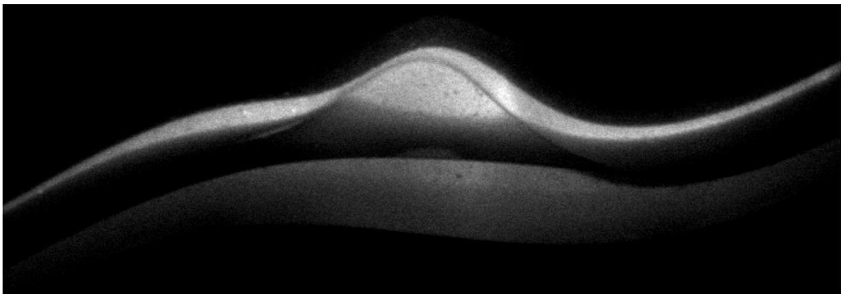
Fig. 1. Side-view of a hump in open channel flow over wavy bottoms detected with the inclined camera. The flow is from the right to the left.
